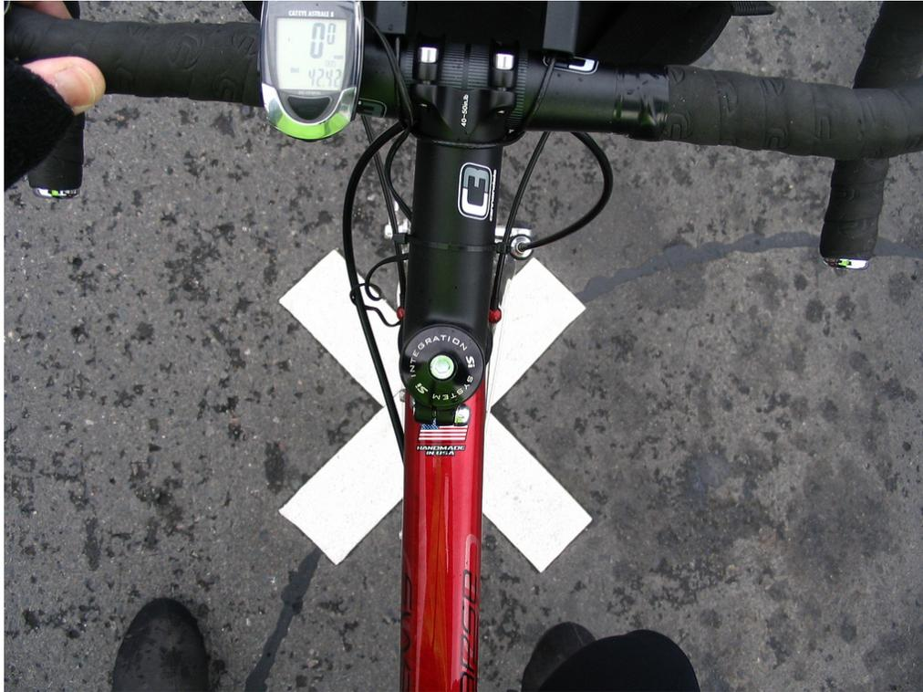
These "X" marks in Bellevue are the locations on the road sensor most sensitive to a cyclist. It allows us to trigger the signal. **Thank you Bellevue!** [Jim Carson]
