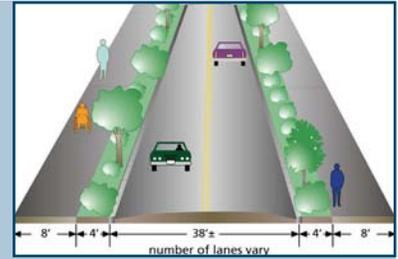
***Diagram illustrating the desired dimensions of an 8 foot-wide pedestrian facility along a major/minor arterial street or downtown minor connection.***
