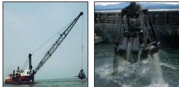
Figure 6: Left to right: typical dredge barge with clamshell bucket, close-up of bucket
