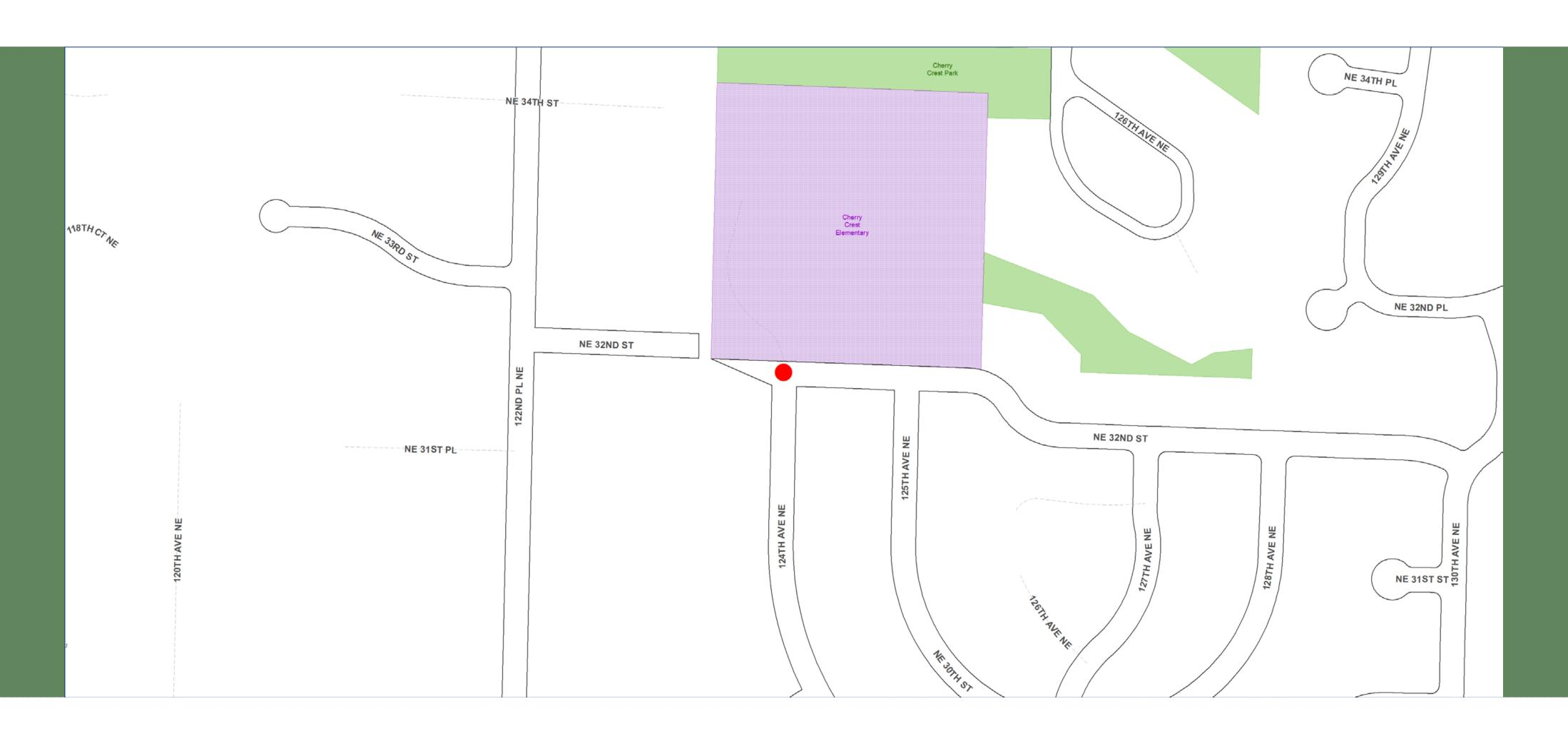
**Description:** This project would enhance the three-leg intersection to encourage stop compliance and a safer pedestrian crossing condition. Includes the installation of a new streetlight on southwest corner of 124th Ave NE and NE 32nd St. Also includes the replacement of existing STOP signs with flashing STOP signs to enhance visibility. Crosswalk paint inside of existing north-south crosswalk would be added.
