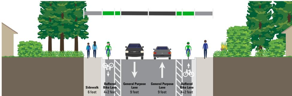
Four-foot bike lanes with two-foot buffers on both sides
