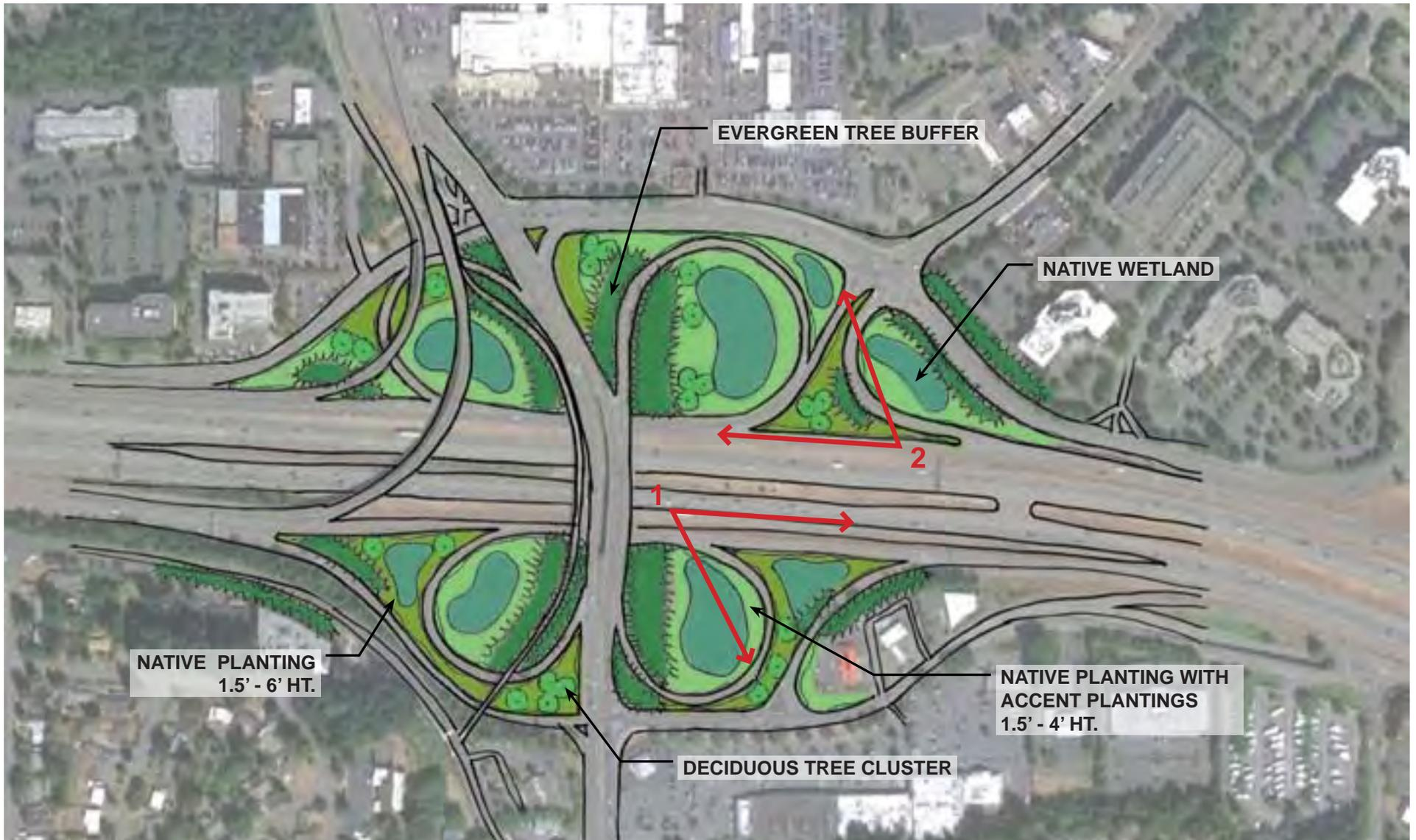
FIGURE D-4 Eastgate Interchange Planting Option B
