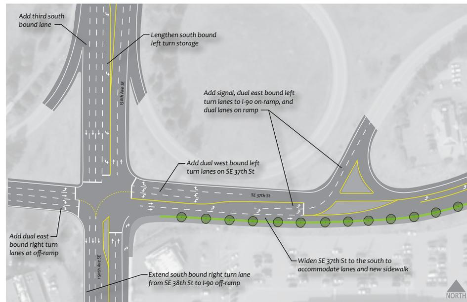
**FIGURE 20** 150th Avenue SE and I-90 Eastbound Off-ramp Intersection Improvement Option (Project I-4: Option A)
