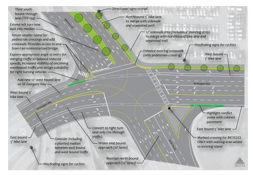
**FIGURE 14** 150th Avenue SE and SE Eastgate Way Signalized Intersection Improvement Option (Project I-2: Option A)
