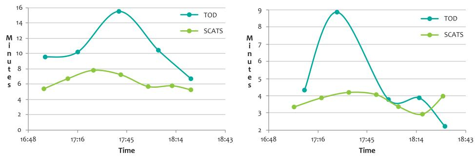
**FIGURE 13** Travel time comparison showing Factoria Boulevard operations with previously used "TOD" time-of-day signal timing plans compared to SCATS traffic control; southbound (left) and northbound (right).
