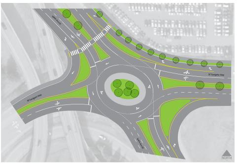
**FIGURE 15** 150th Avenue SE and SE Eastgate Way Roundabout Improvement Option (Project I-2: Option B)
