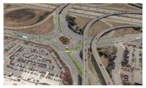
**FIGURE 16** WSDOT Simulation Model of Roundabout Improvement Option (Project I-2: Option B; looking south)
