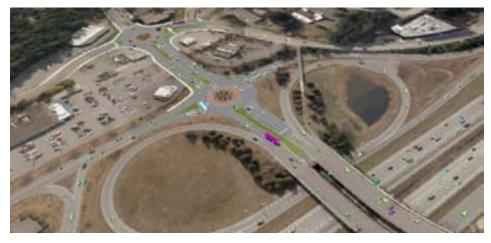
**FIGURE 22** WSDOT Simulation Model of Roundabout Improvement Option (Project I-4: Option B; looking south)
