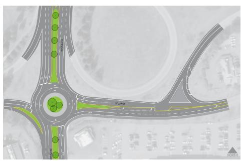
**FIGURE 21** 150th Avenue SE and I-90 Eastbound Off-ramp Roundabout Improvement Option (Project I-4: Option B)
