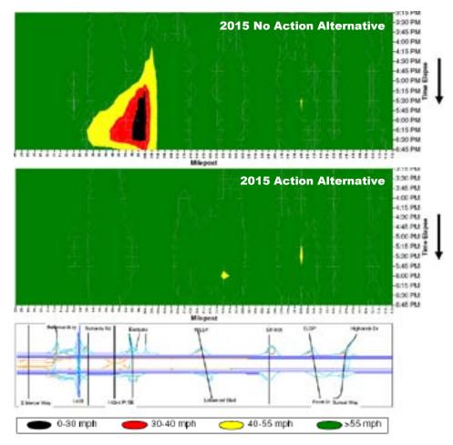
**FIGURE 26** WSDOT study results showing I-90 eastbound speed profile with and without auxiliary lane improvement. In the 2015 action alternative, vehicles will have more space to enter the mainline traffic at the Eastgate interchange resulting in a smoother merge and less congestion at this location.
