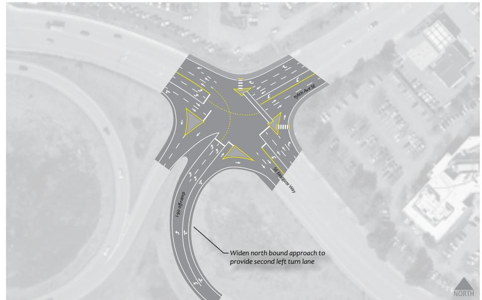
**FIGURE 17** 156th Avenue SE and SE Eastgate Way Intersection Improvement Option (Project I-3: Option A)
