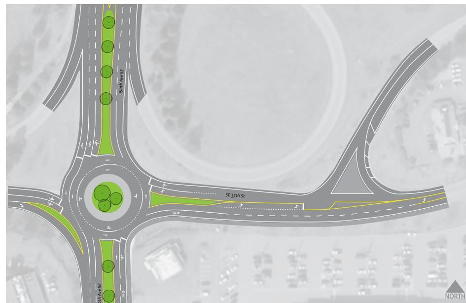
**FIGURE 21** 150th Avenue SE and I-90 Eastbound Off-ramp Roundabout Improvement Option (Project I-4: Option B)
