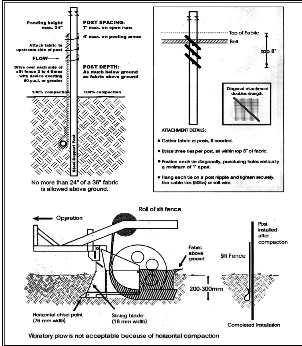
**Figure 4.2.13 – Silt Fence Installation by Slicing Method**
