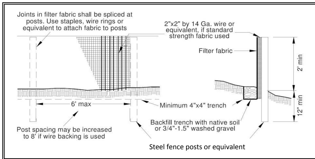
**Figure 4.2.12 – Silt Fence**
