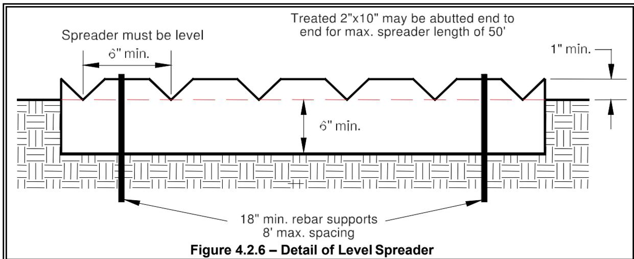
**Figure 4.2.6 – Detail of Level Spreader**
