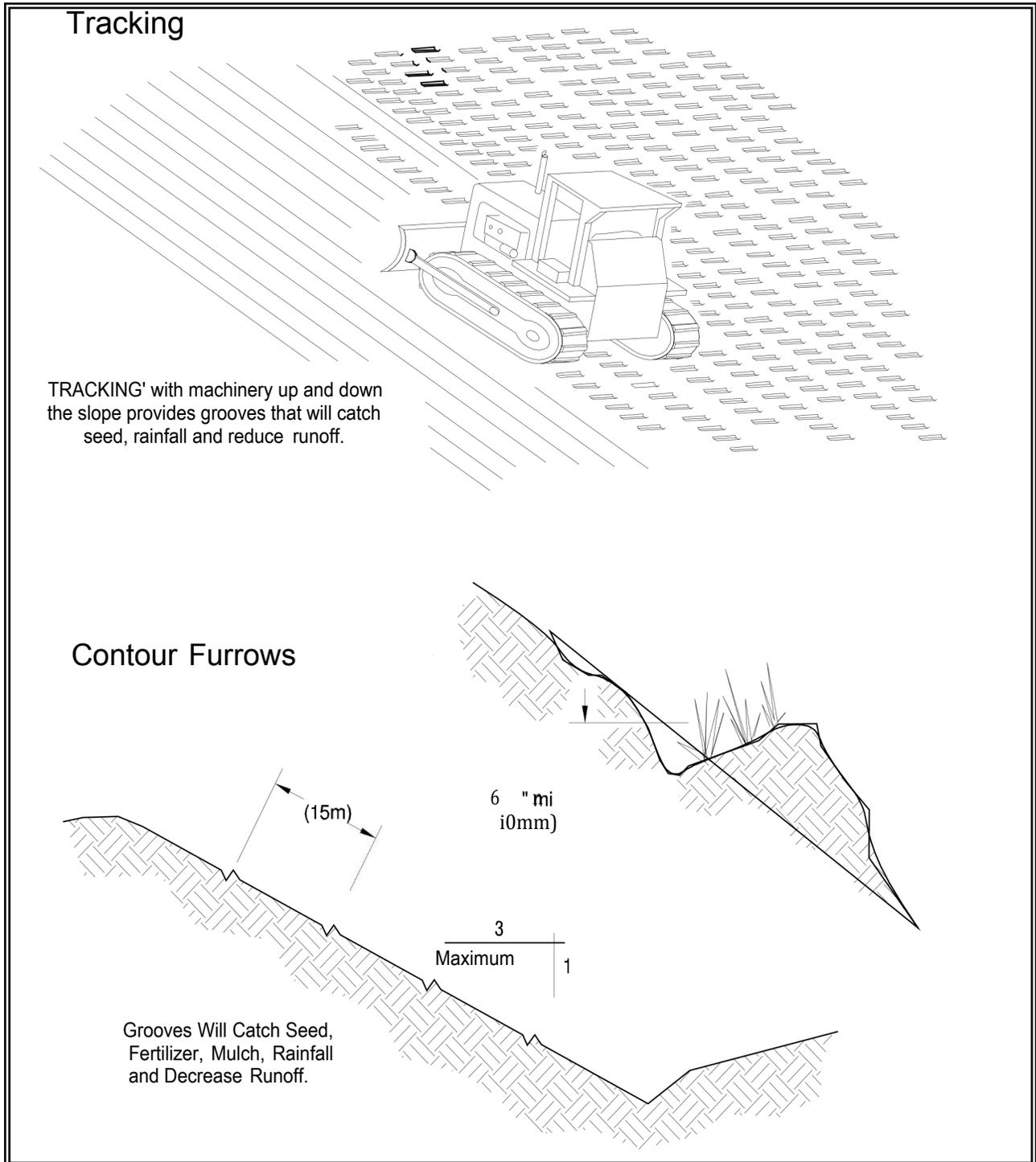
Figure 4.1.5 — Surface Roughening by Tracking and Contour Furrows
