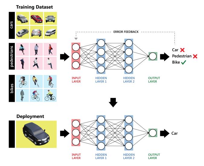
Figure 9: Deep Neural Network algorithms learn from off-line training inputs to detect subtle variations among different objects and then make data-driven predictions of observed data during real-world deployment.
