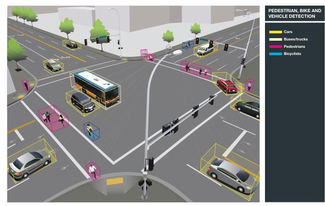
*Figure 5:* The technology development partnership has already demonstrated the capability of leveraging the city's traffic camera system to accurately detect and differentiate pedestrians, bicyclists and cars.
