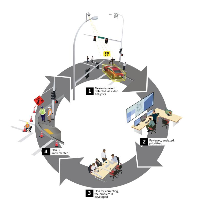
*Figure 3:* The algorithms under development aim to create a 24/7 predictive crash analysis system that flags near-misses in real-time, enabling public works departments to implement safety countermeasures before someone gets hurt.
