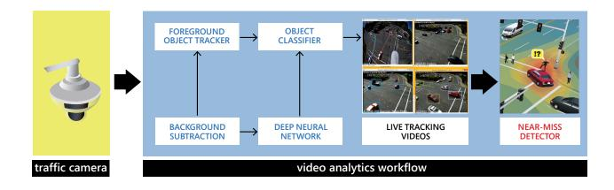
*Figure 4:* The system tracks objects on live feeds from a city-wide camera installation, classifying objects into vehicles/pedestrians/bicycles using a deep neural network, and flagging near-miss events.
