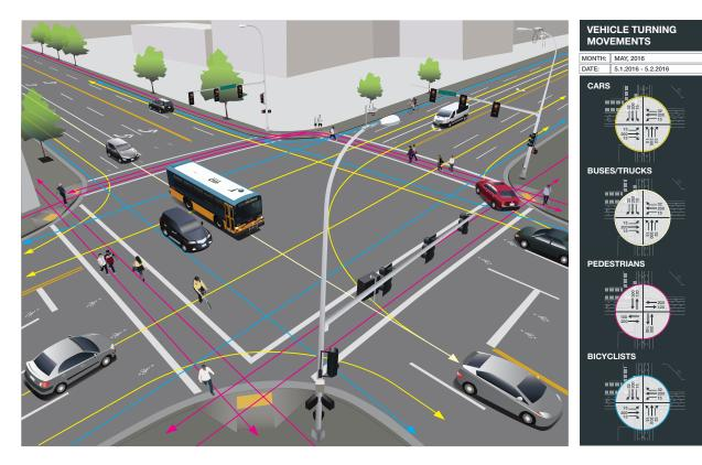
Figure 6: The city's traffic camera system also can be used to count and track the movements of pedestrians, bicyclists and cars.
