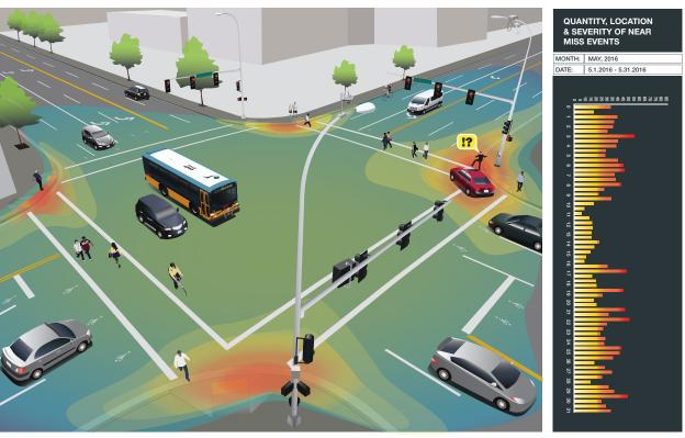
Figure 8: Identifying near-miss hot-spots will allow traffic planners and engineers to pinpoint problems and evaluate the effectiveness of countermeasures.
