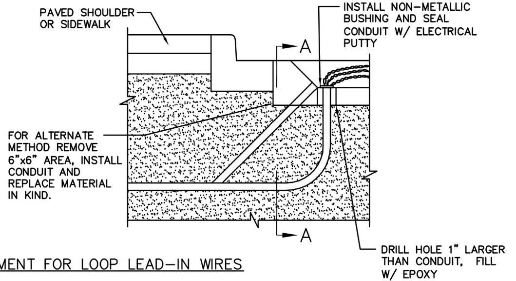
TYPICAL CONDUIT PLACEMENT FOR LOOP LEAD-IN WIRES
