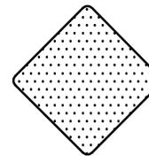
18" X 18" YELLOW HIGH INTENSITY TYPE 1 OBJECT MARKER PLACED IN TRAFFIC CIRCLE FOR EACH APPROACH. ALL SIGNS TO BE MOUNTED ON SINGLE POST. LOCATION TO BE DETERMINED BY ENGINEER. SIGN HEIGHT: 5' FROM BOTTOM OF LOWER SIGN TO BARK MULCH.
