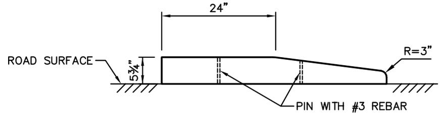
ELEVATION - TYPE A NOSING AND C NOSING
