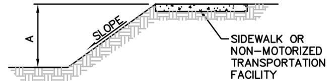
SAFETY RAILING WARRANTED WHEN: SLOPE IS STEEPER THAN 2H:1V AND DIMENSION "A" IS  $\geq$  1 FOOT
