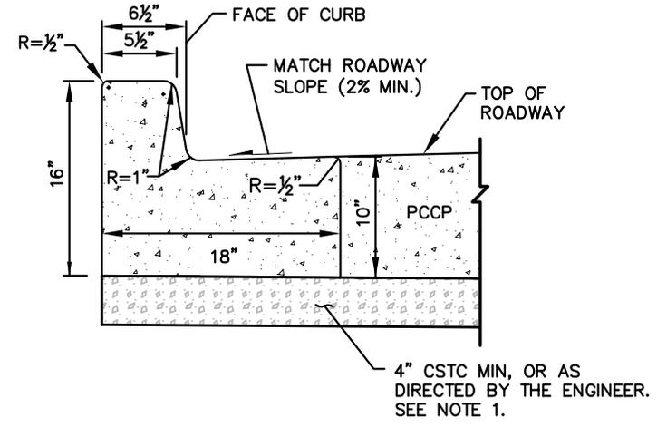
MODIFIED CEMENT CONCRETE TRAFFIC CURB & GUTTER
