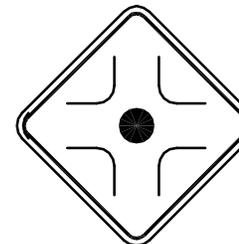
30" X 30" BLACK ON YELLOW PLACED 75' TO 100' BACK FROM TRAFFIC CIRCLE ON EACH APPROACH. SEE STD. DWG. TE-21B FOR POST TYPE AND INSTALLATION.
