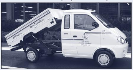
Made by Miles Electric Vehicles of Santa Monica, Calif., the truck has six large batteries and plugs into a regular outlet. Charged overnight, it is ready to roll in the morning.
