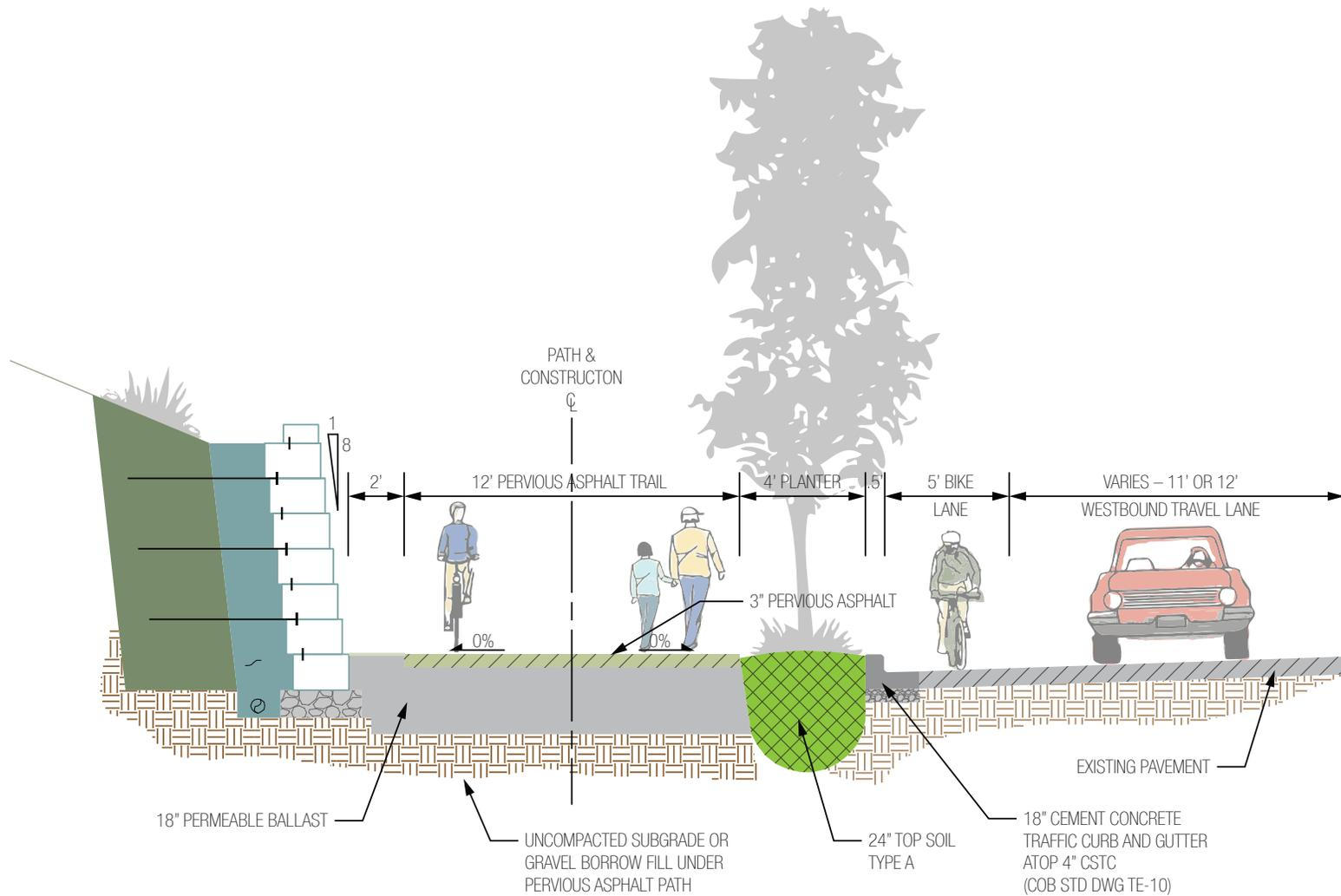
**FIGURE 43** Trail section A-A (not to scale).
