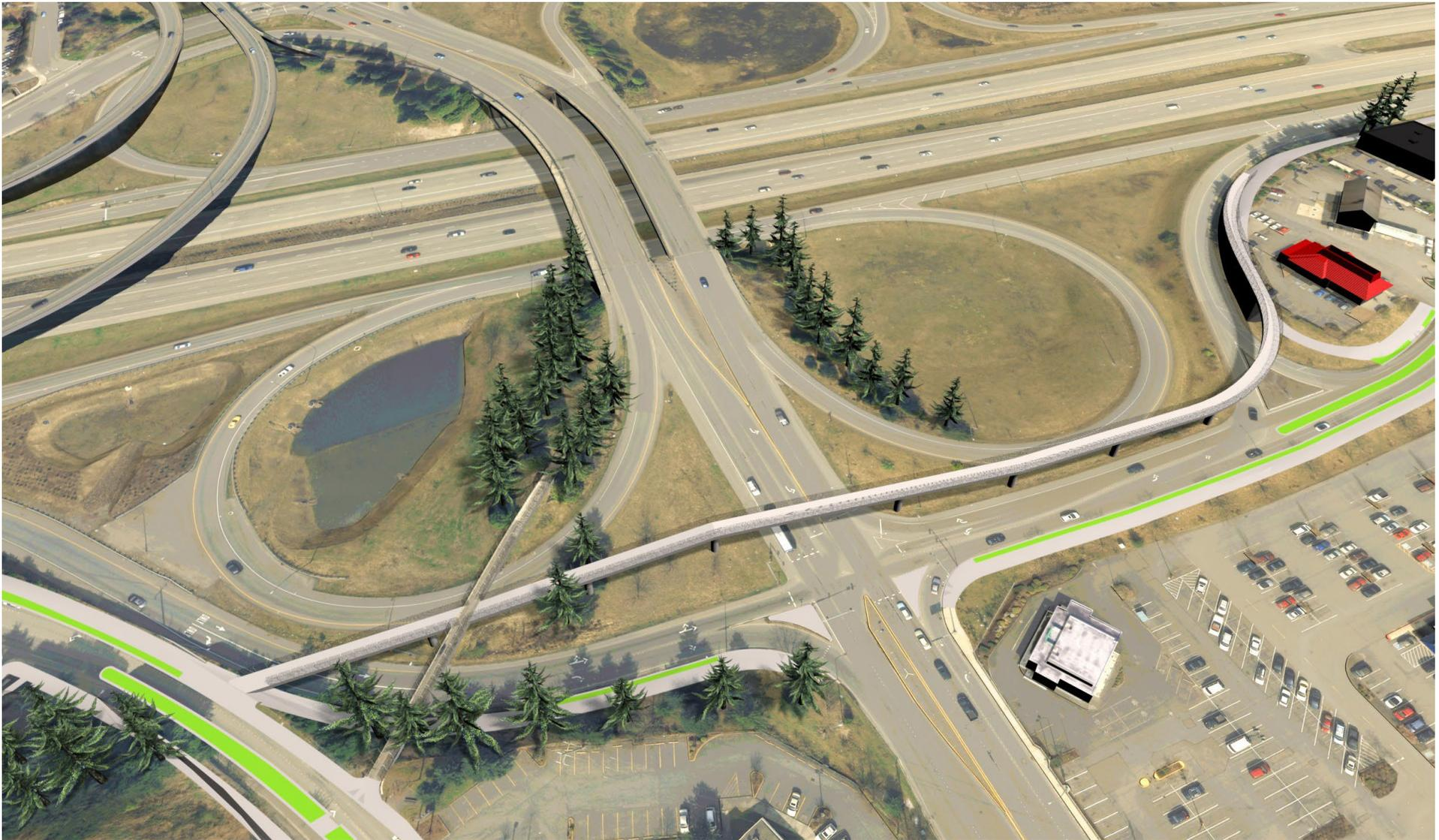
**FIGURE 29** Photovisualization of the bridge crossing over 150th Ave SE as a long range alternative to bypass the busy intersection of 150th Ave SE and SE 37th St (looking north).
