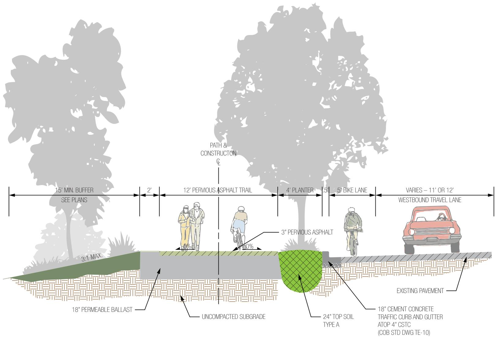
**FIGURE 44** Trail section B-B (not to scale).
