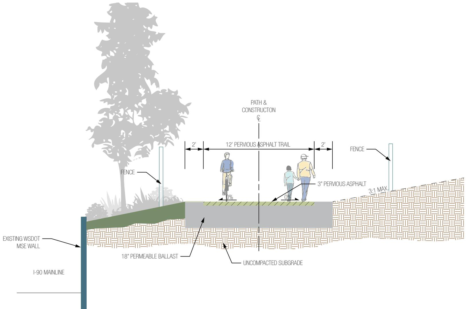
**FIGURE 47** Trail section E-E (not to scale).
