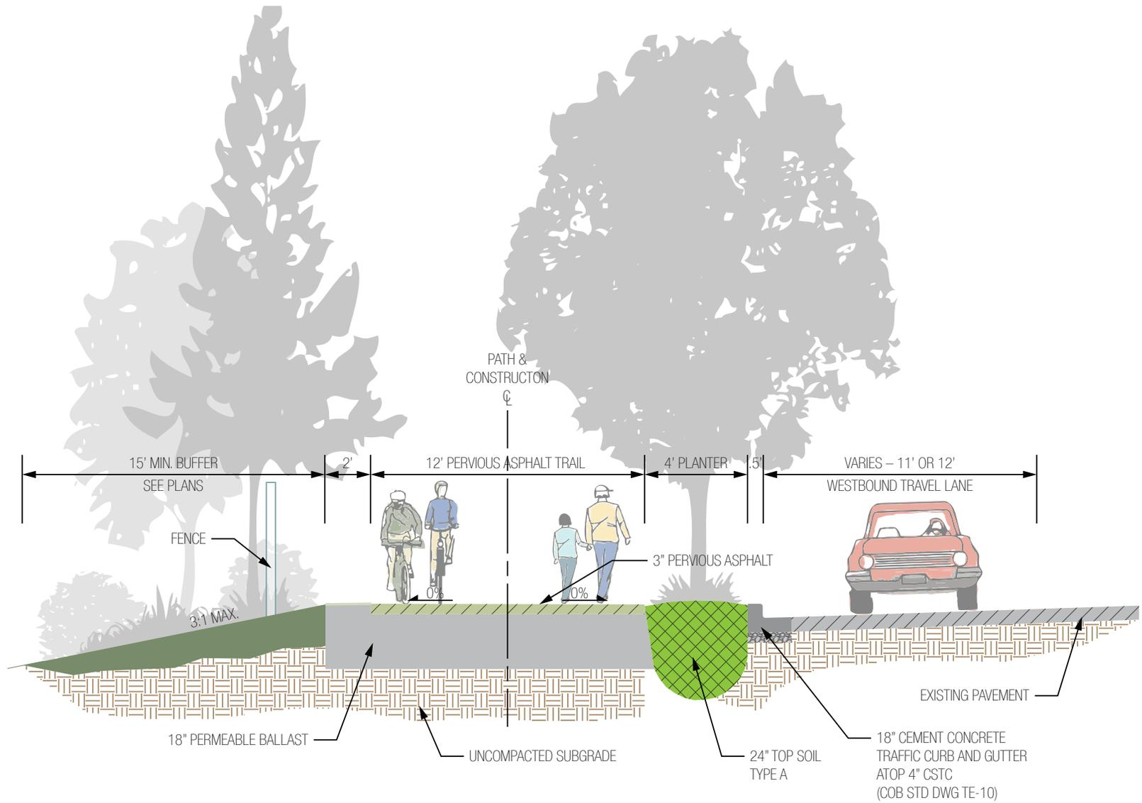
**FIGURE 45** Trail section C-C (not to scale).
