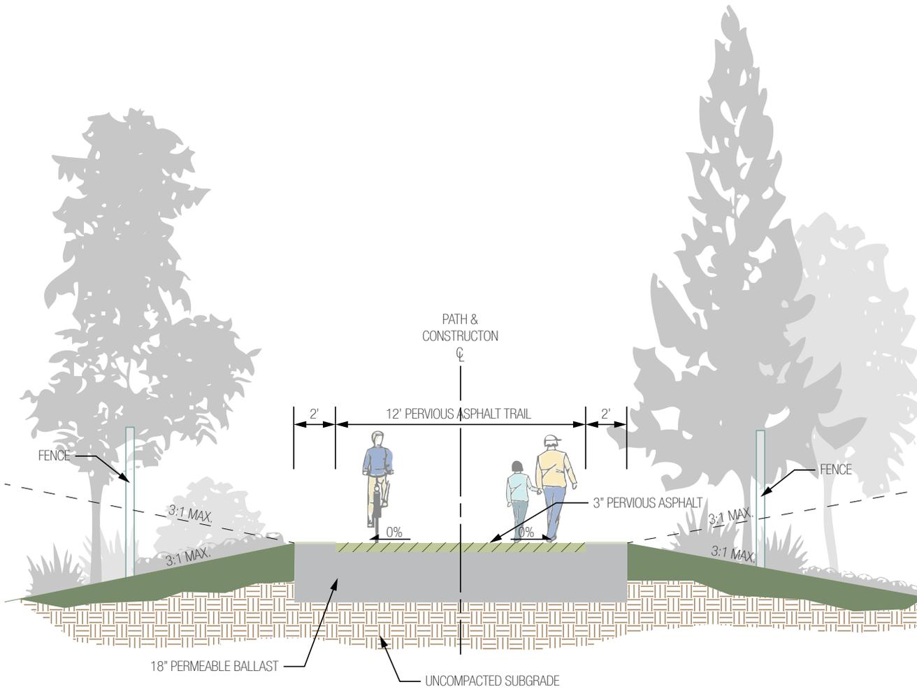
**FIGURE 49** Trail section G-G (not to scale).
