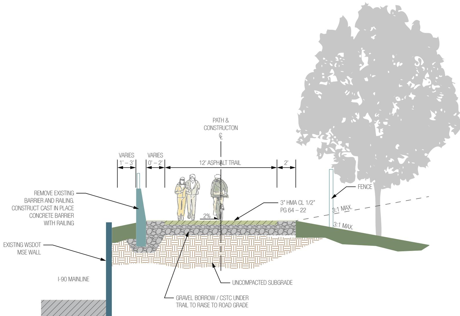
**FIGURE 48** Trail section F-F (not to scale).
