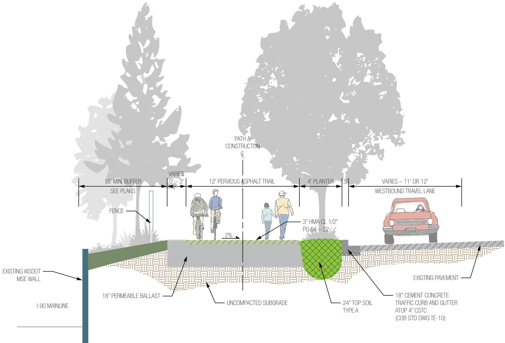
**FIGURE 46** Trail section D-D (not to scale).
