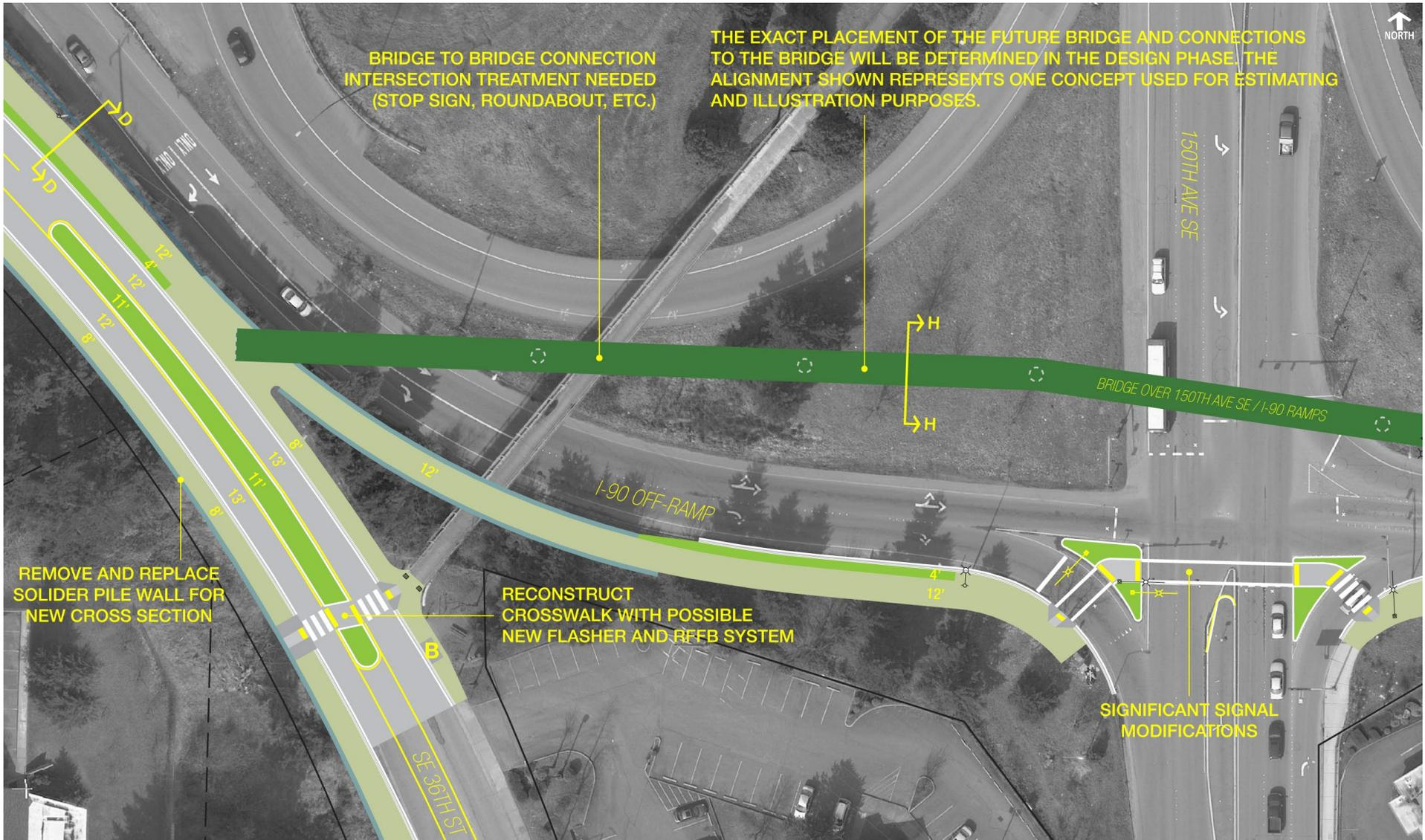
**FIGURE 27** At grade trail and bridge crossing over 150th Ave SE at the I-90 Off-Ramp.
