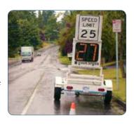
on a reader board. Like the radar dolly, the goal is to heighten drivers' awareness of both the speed at which they are traveling and the posted speed limit. This encourages drivers to adjust their speeds, if needed.
