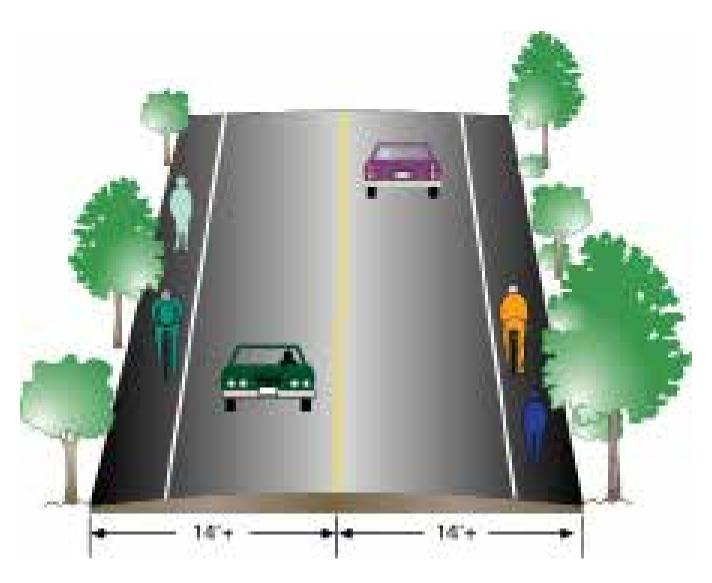
Lane striping can help define the roadway alerting drivers, cyclists, and pedestrians to the correct travel lanes.
