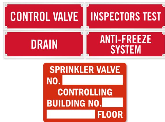
The installing contractor shall also identify a hydraulically designed sprinkler system with a machine engraved weatherproof metal, or rigid plastic sign secured to the riser it serves with corrosion resistant wire, chain, or other approved means. Such signs shall be placed at the alarm valve, dry valve, pre-action valve, or deluge valve supplying the corresponding hydraulically designed area.
