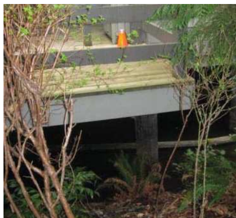
Figure 6-19: Accelerometer Location on top of a Pile (Orange Cone)
