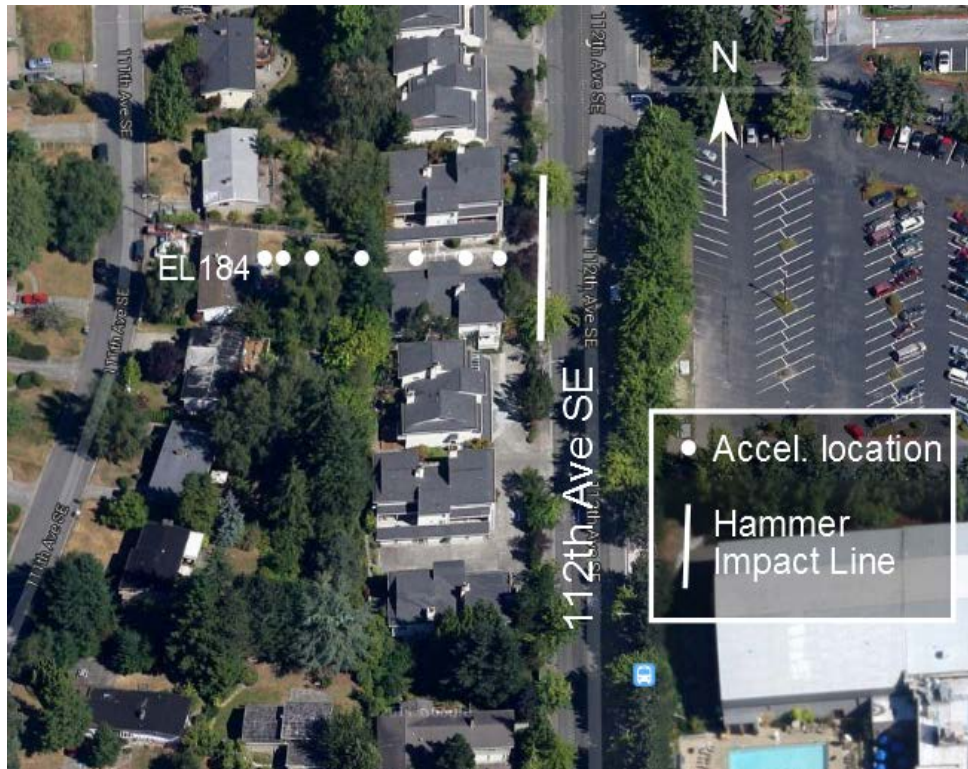
Figure 6-1: Measurement Diagram for Surface Vibration Propagation Test at EL184
