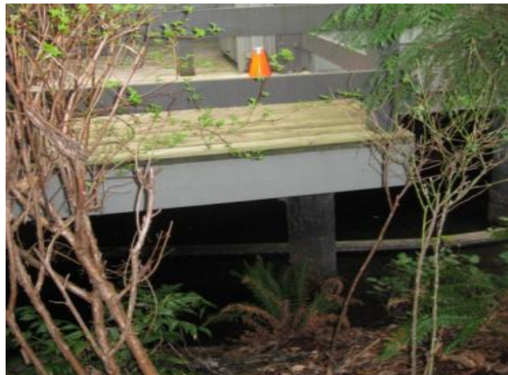
Figure 6-19: Accelerometer Location on top of a Pile (Orange Cone)
