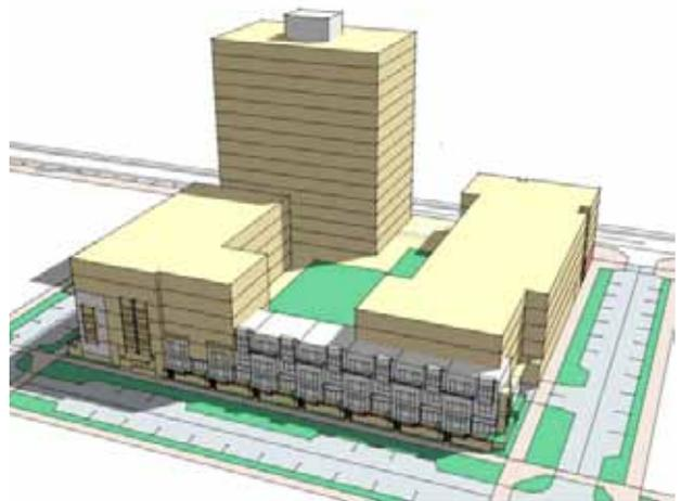
Figure 3.7 This site combines both mid-rise and tower building forms. Parking is located to the interior and may be shared between uses. Larger sites allow for a more efficient parking geometry.
