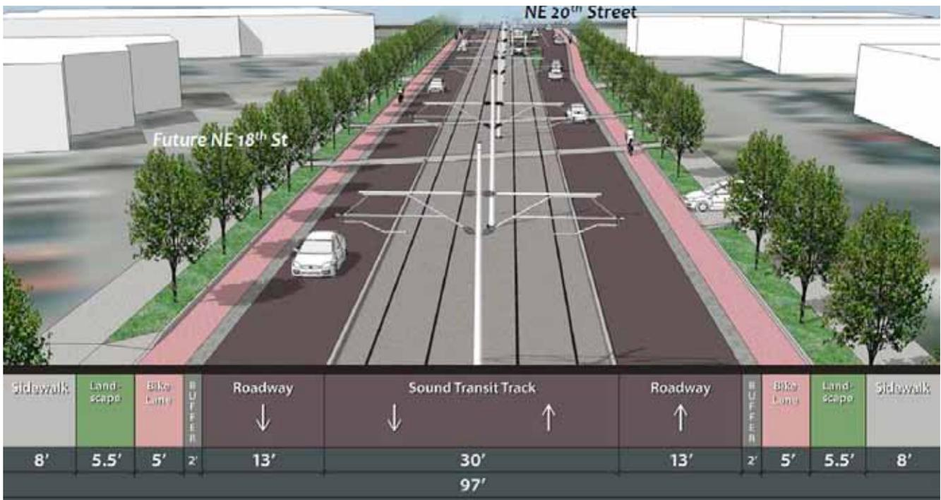
Figure 5.11 136th Place NE planned cross section
