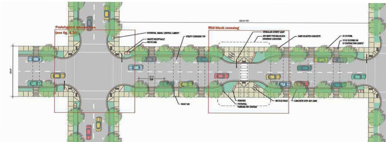
Figure 5.13 Local Street Section and Plan
