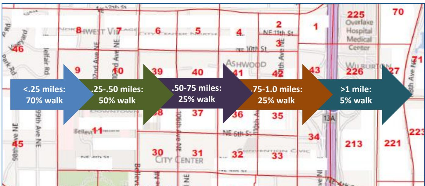
**Figure 1.** Distance Methodology for Internal Walk Trip Calculation
