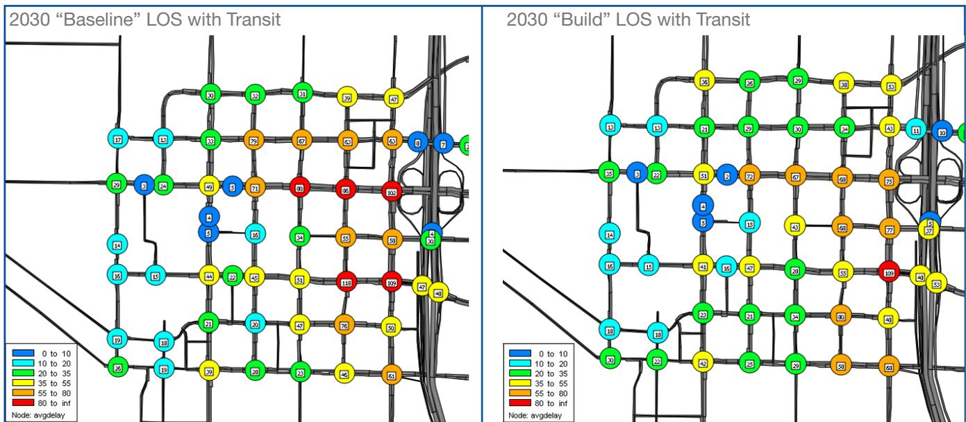
**Figure 6.** Dynameq Modeling Output - Vehicle Level-of-Service (Delay)
