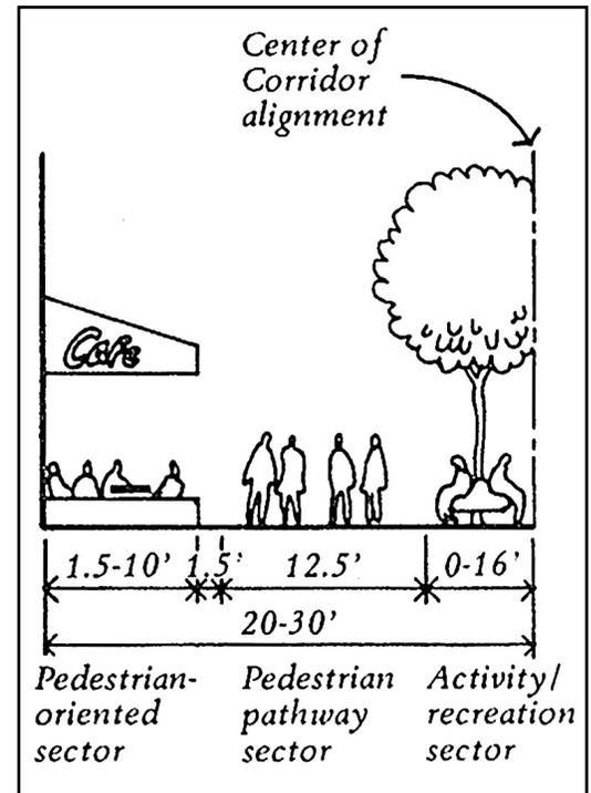
Figure 19. Building the Pedestrian Corridor by Halves
