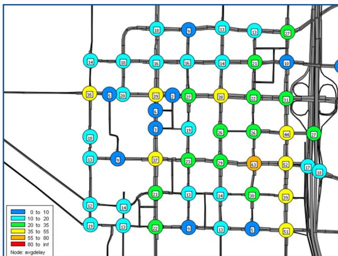
**Figure 5.** Intersection 2010 Level-of-Service (Delay)
