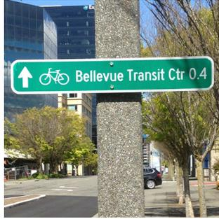
signage at decision points that identifies the direction and distance to specific destinations, and confirmation signage after the turn to point the bicycle rider in the right direction.
