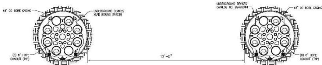
Figure 3-13 XLPE Typical Jack and Bore Detail
