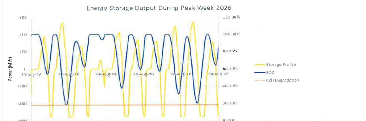
Figure 11: Output of the Complete Solution during the peak week, 549MW/5,500MWh (10.0-hour system)
