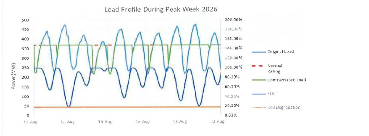
Figure 10: The Complete Solution during the peak week, 549MW/5,500MWh (10.0-hour system)
