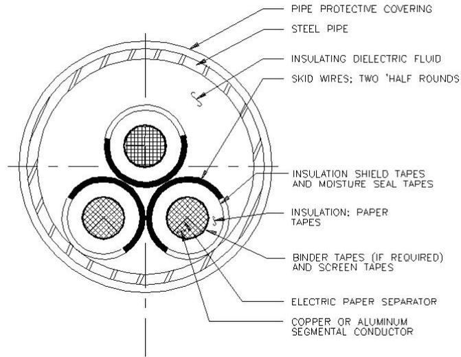
**Figure 2-11 Typical Cable and Cable Pipe Cross-Section**
