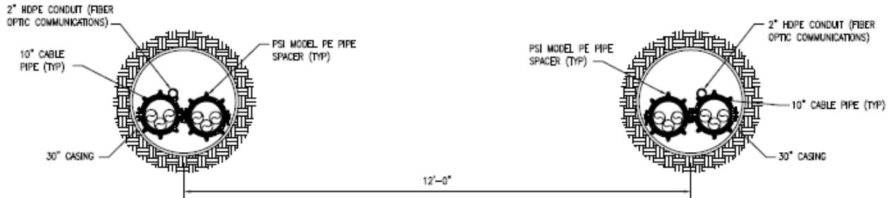
Figure 3-16 HPFF Typical Jack and Bore Detail
