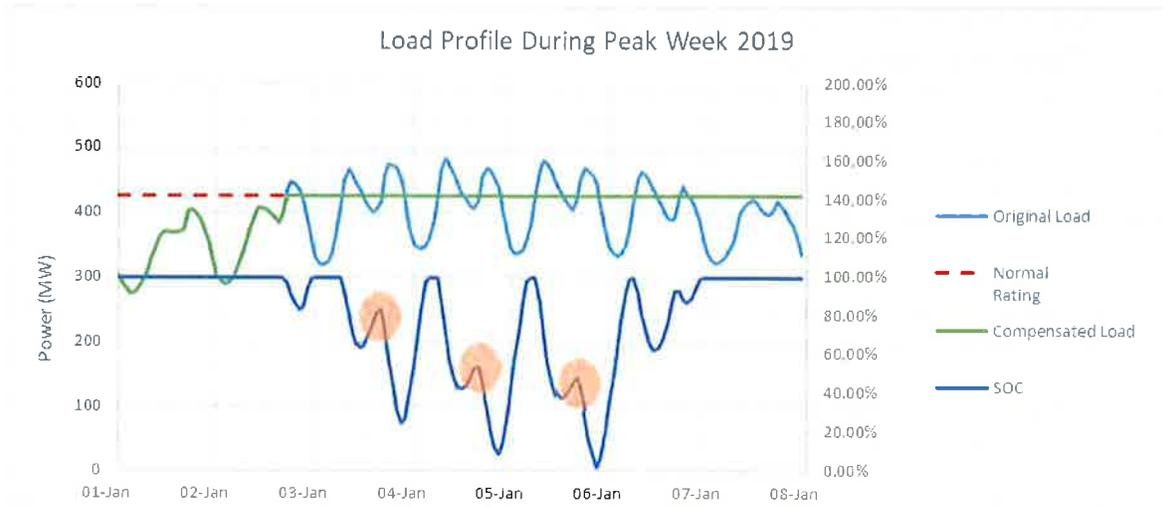
Figure 3: The Interim Solution using the updated methodology during the peak week: 290MW/1,689MWh (5.8-hour system) – circles highlight intra-day recharging
