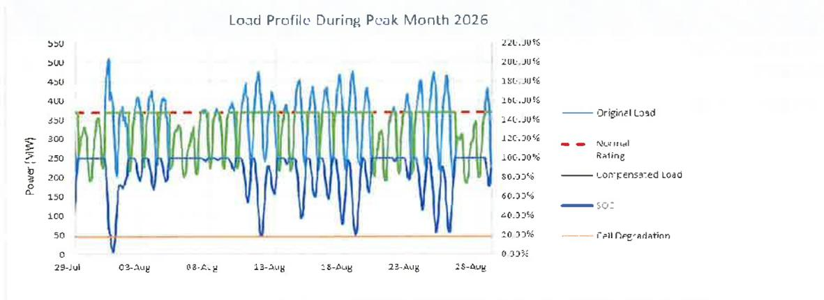
Figure 12: Performance over peak summer month, 549MW/5,500MWh (10.0-hour system)
