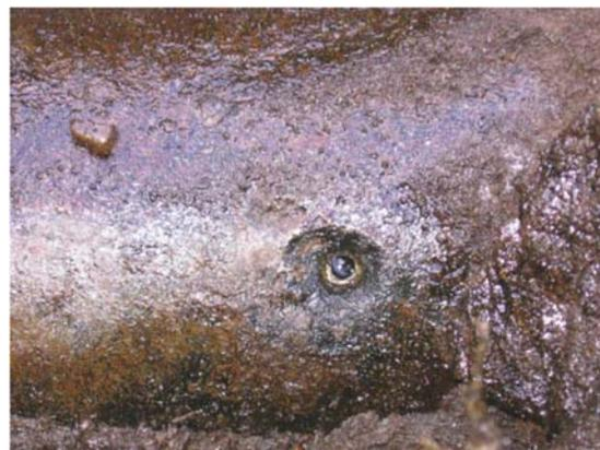
Representative photograph from PHMSA report showing hole in a pipe wall caused by electrical fault (not Olympic Pipeline system)
