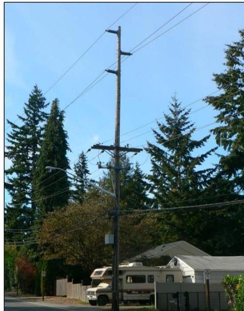
Utility pole carrying transmission wires (top section), distribution wires (middle section), and telecom wires (lower section)
