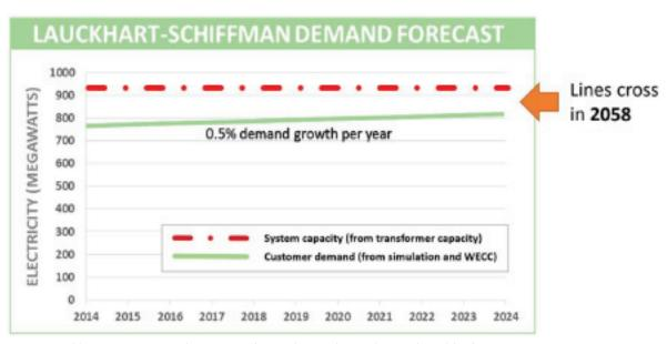
Figure 5: Alternative Demand Forecast shows slower demand growth and higher system capacity (based on "winter emergency" transformer ratings).
