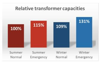
Figure 7: Ratings for different scenarios, normalized to Summer Normal rating.
