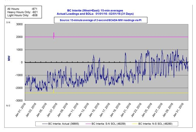
The dark blue line shows energy transfers between the Puget Sound and British Columbia updated every 15 minutes during the month of January 2016. When the line is below the axis, electricity is flowing from Canada to the US, as it did for most of the first three weeks in January. As temperatures warmed, electricity began flowing back and forth between the two countries (but still mostly southward).
