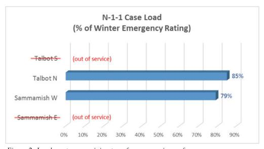
Figure 2: Loads on two remaining transformers are in a safe range.
