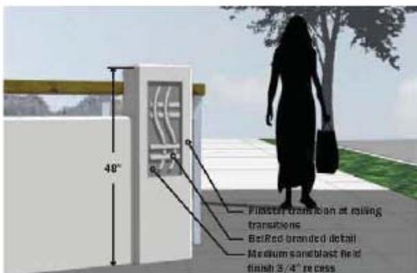
Figure 7 – Concrete Pilaster
