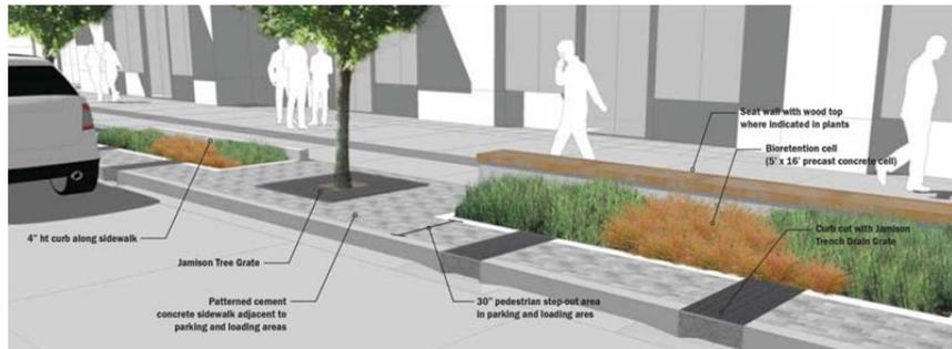
Figure 12 – Stormwater Bioretention Cells
