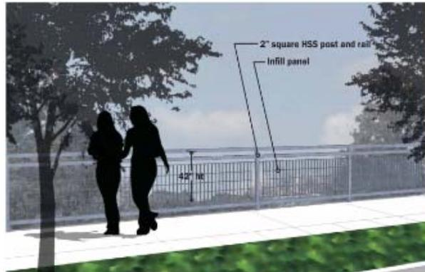
Figure 9 – Typical Pedestrian Railing
