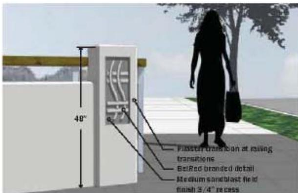
Figure 7 – Concrete Pilaster
