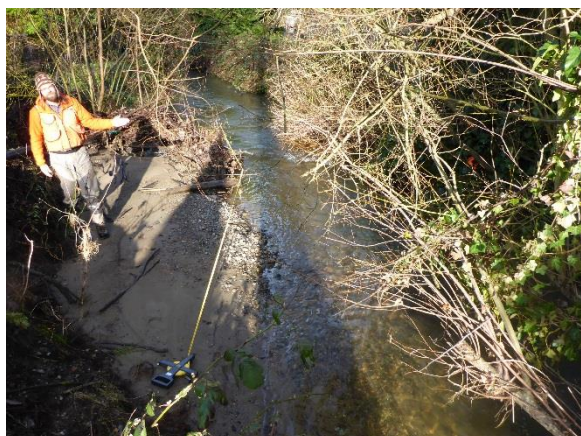
Figure 5: Location of anomalously wide bankfull width 125 ft above Upper Skagit Key. The channel is anomalously wide at this location due to sedimentation above the downstream obstruction.
