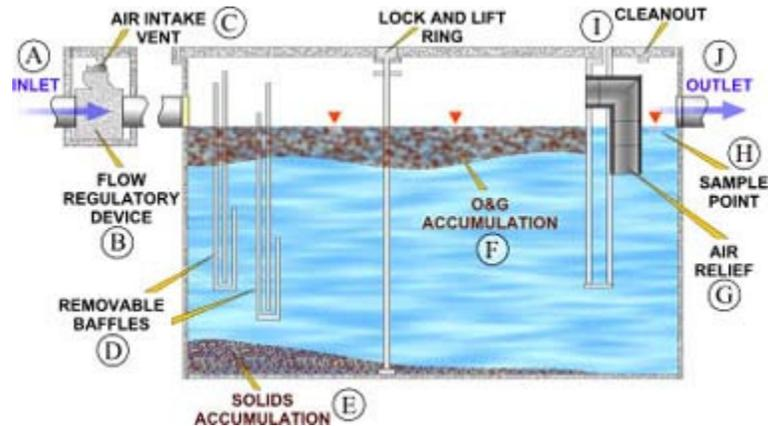
**How a Grease Interceptor Works (see diagram following table).**
