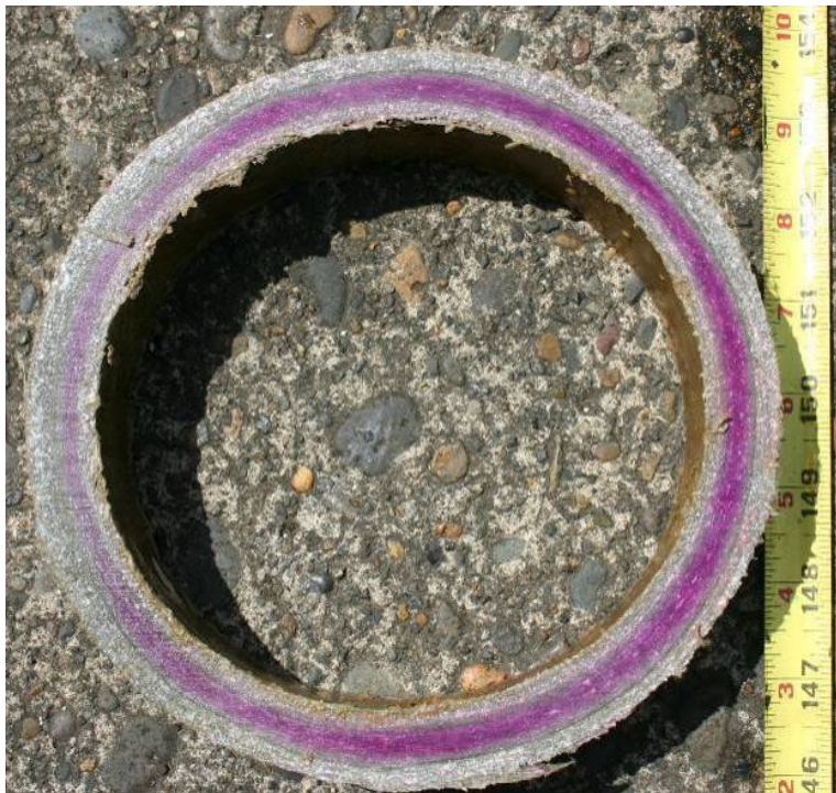
Figure 8-3: Cement Mortar Leach Test on AC Main
