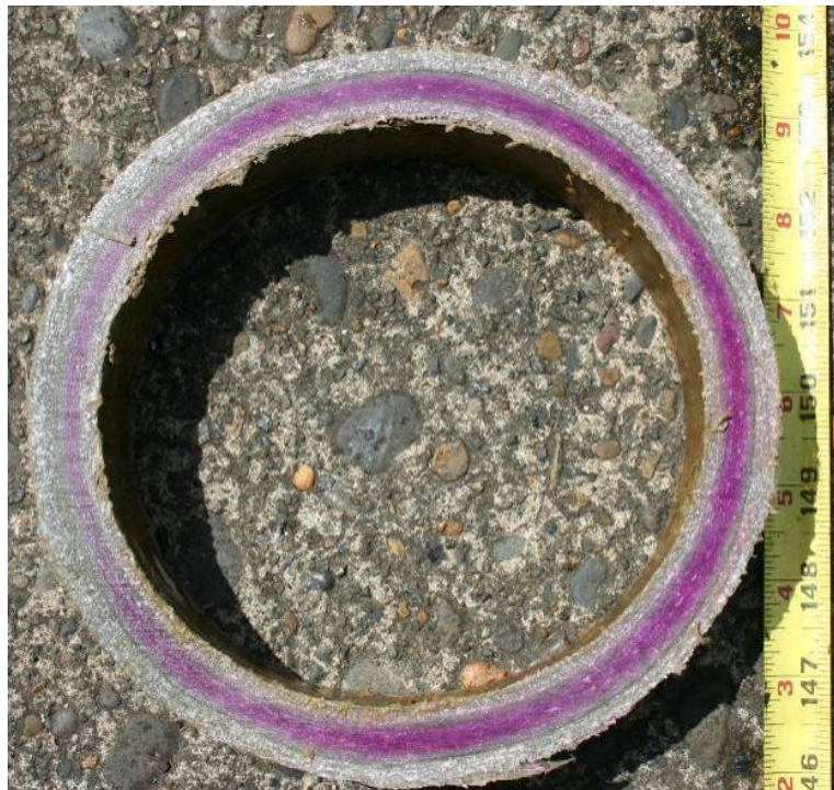
Figure 8-3: Cement Mortar Leach Test on AC Main
