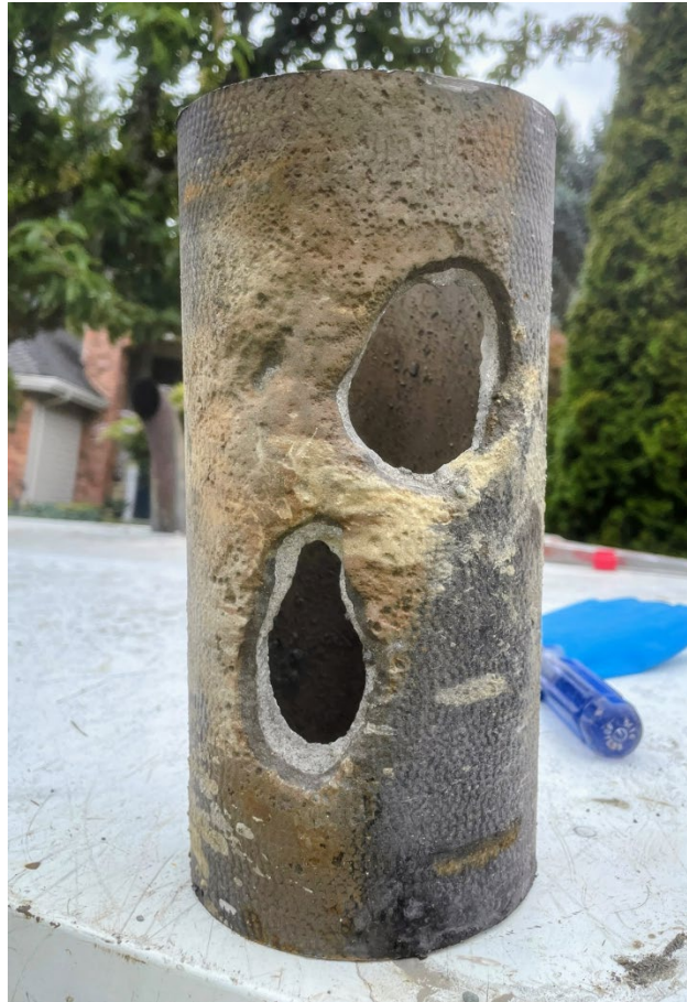
Figure 8-4: Corroded Ductile Iron Water Main
