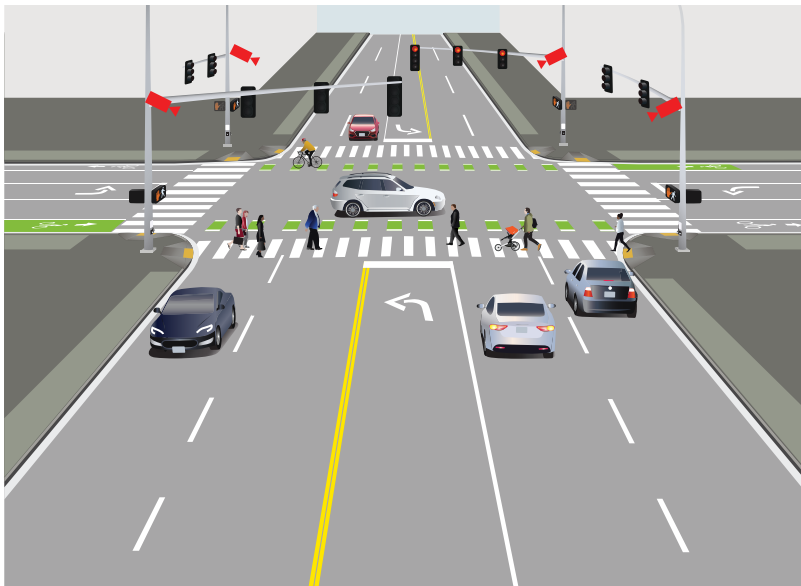
Figure 12. Passive Pedestrian Detection Phase Extension Use Case
