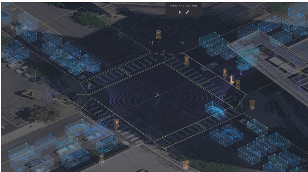
Figure 19: LiDAR sensor capabilities on our RTSSI project allows the traffic signal system to detect every pedestrian and their associated walk speed. This, in turn, allows the traffic signal system to apply real-time interventions such as additional walk time or phase extensions to mitigate real-time risks to vulnerable road users.
