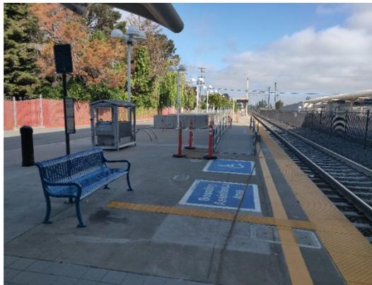
**821.3.21.2** The waiting area must be 6 feet wide and extend the full depth of the platform, except where the platform edge detectable warning tile and the tactile wayfinding path are located. See Figure 821-2.
