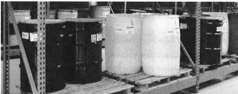
Figure 1: Drums containing dangerous waste, properly labeled and stored safely while waiting for disposal or treatment by generator.
