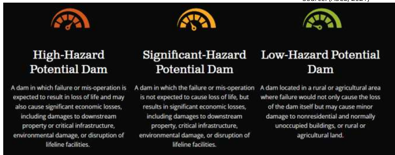
Figure 8-1. Dam hazard potential classifications
