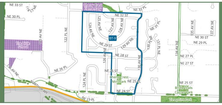
**Description:** This project would assist in maintenance of the approximately sixty (60) existing post-top street lights in the Cherry Crest Neighborhood. The posts would be cleaned, repainted, and the globe system, including the lens, would be replaced with new tops.
