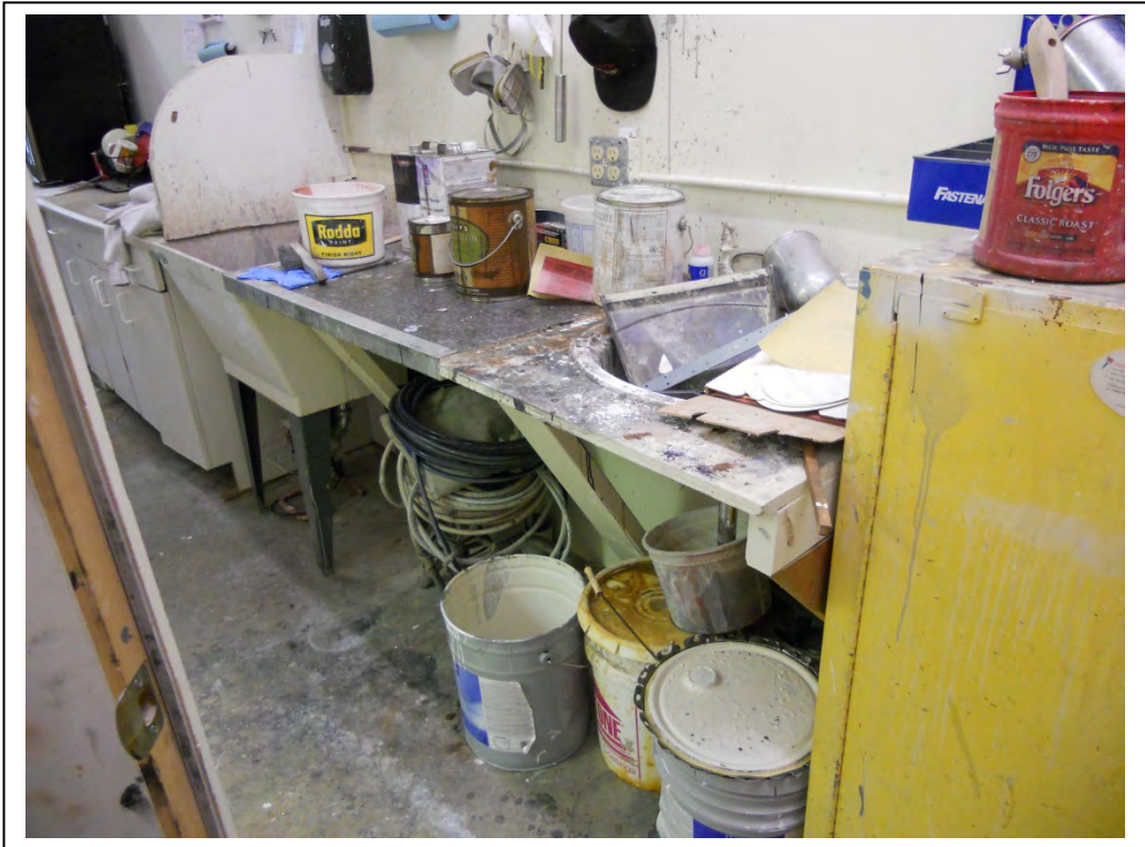
Photo 11: Extensive staining and improper chemical storage in office hallway of The Wall Doctor, Inc.
