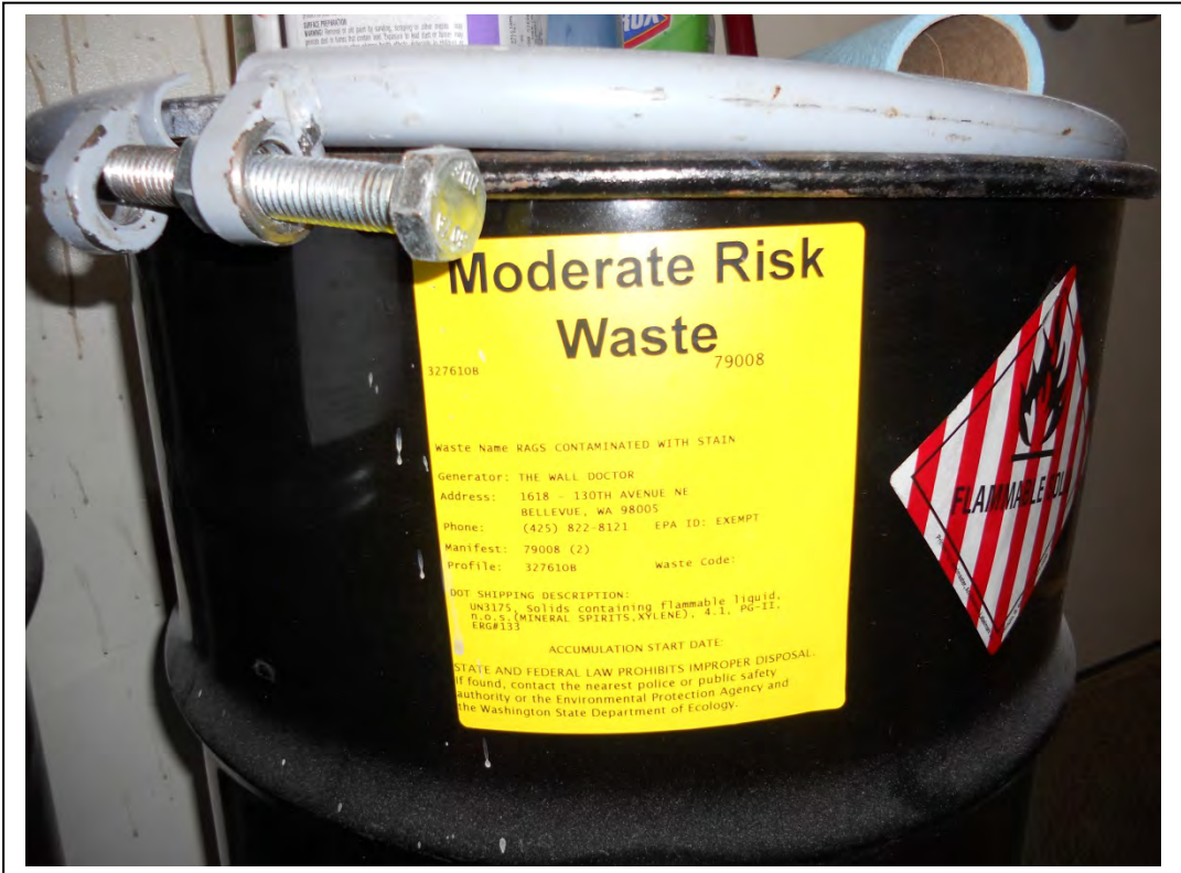
Photo 10: Waste drum with unsecured lid.
