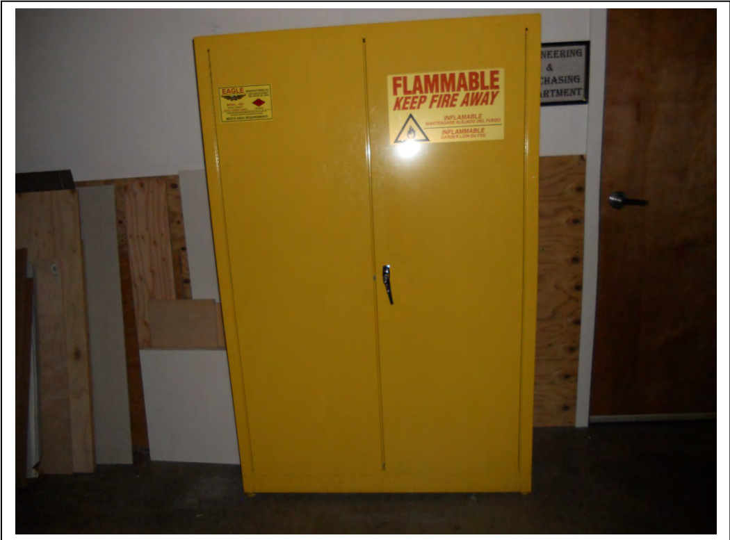
Photo 11: Flammable chemical storage cabinet noted in warehouse area.
