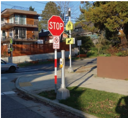
2 Separate RRFB activation button for bicyclists at the street curb
