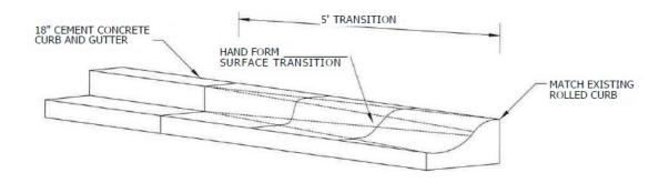
There needs to be 5 feet of transition in between the existing rolled curb and the concrete curb and gutter. This transition needs to be a hand formed surface transition.
