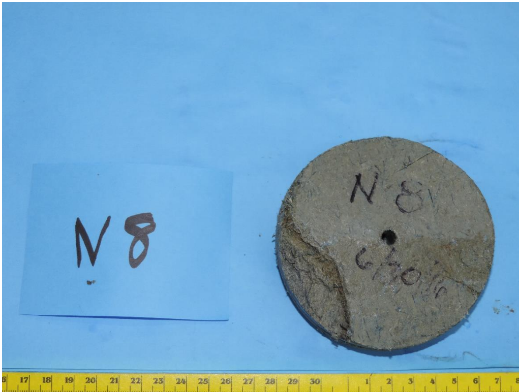
Overall view of sample N-8. Note the area that has chipped off on the OD.
