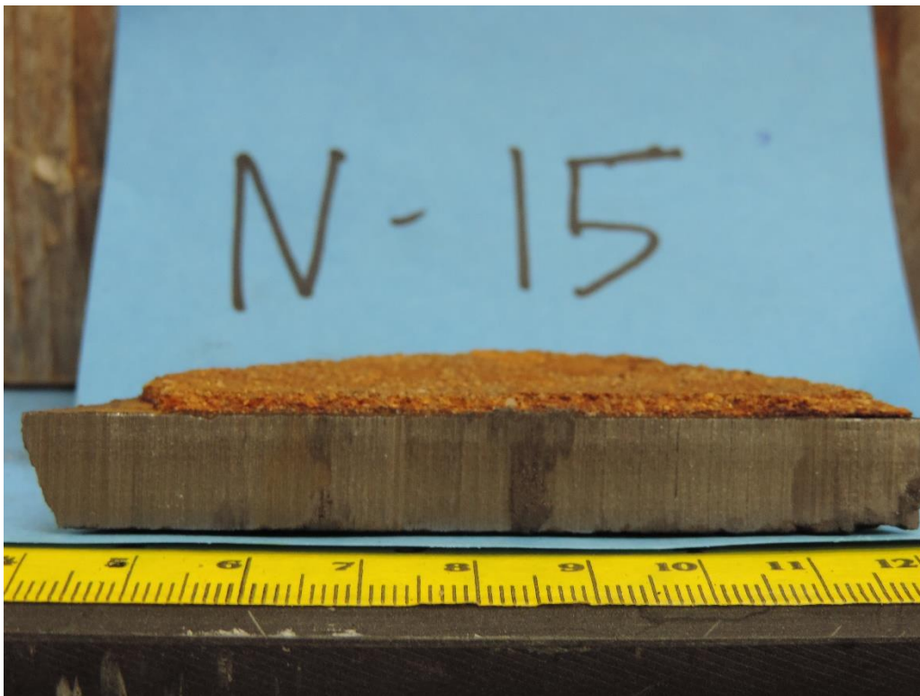
Close up of the cross section of sample N-15. The pH testing indicated the cement layer was acidic, but due to the heavy iron staining an accurate reading could not be obtained.
