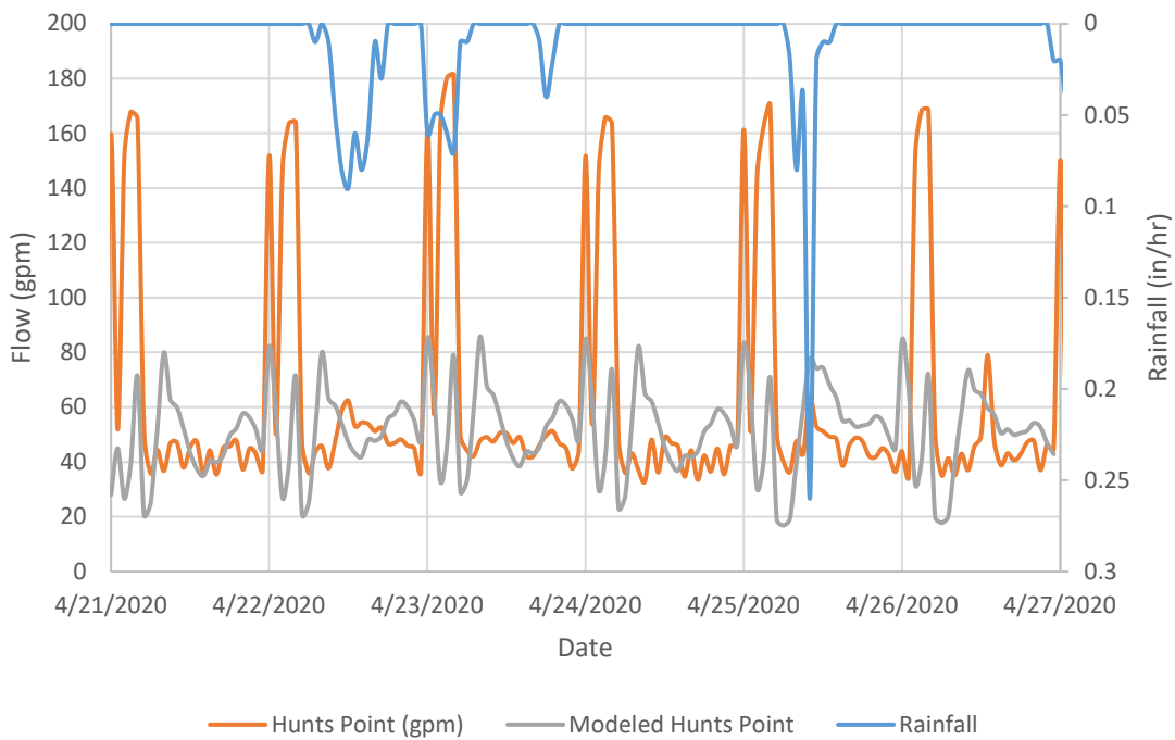
Hunts Point Storm 3 WWF Calibration
