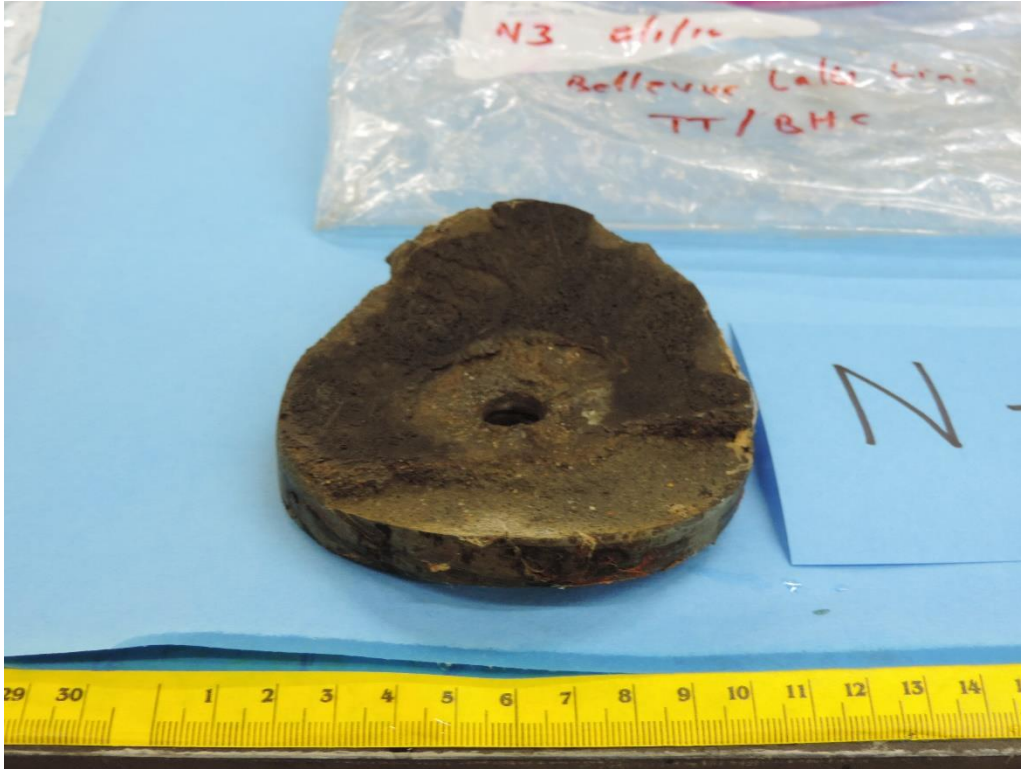
Close up of the inside of sample N-3 with a chipped cement layer.
