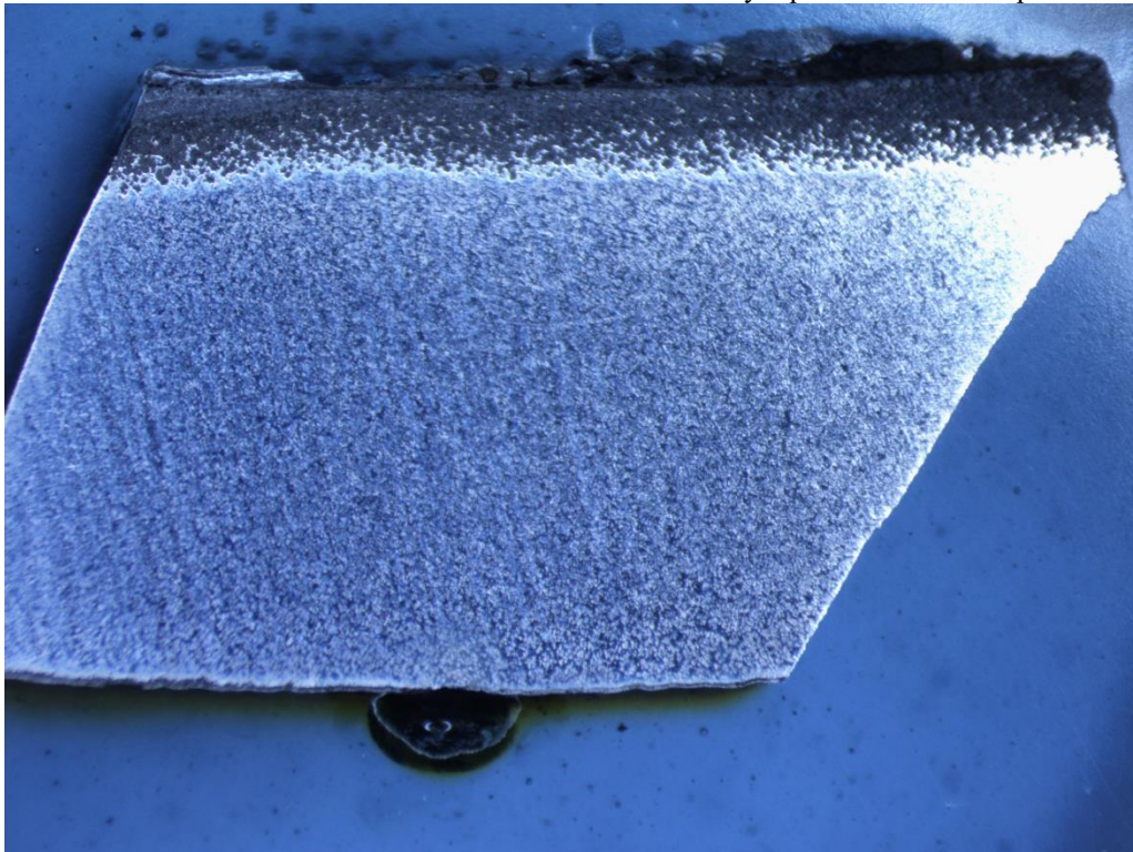
7x view of the cross section from sample N-16. Note corrosion has initiated at the inside surface in the absence of cement.
