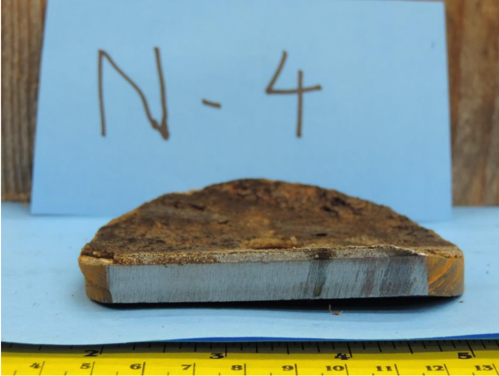
Close up of the Ph and phenolphthalein tested cross section from N-4. An acidic pH was detected, except directly above the cast iron pH was neutral.
