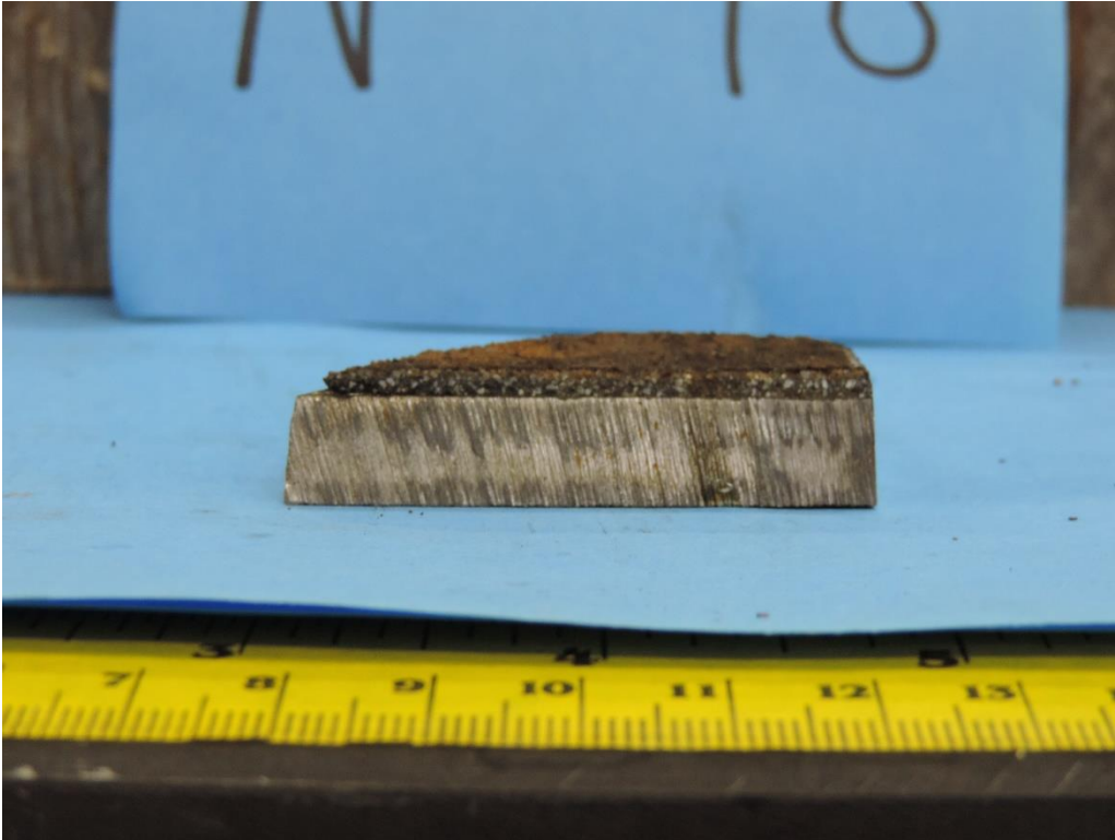
Cross section of sample N-18. The cement layer had darkened sufficiently so an accurate pH could not be measured.
