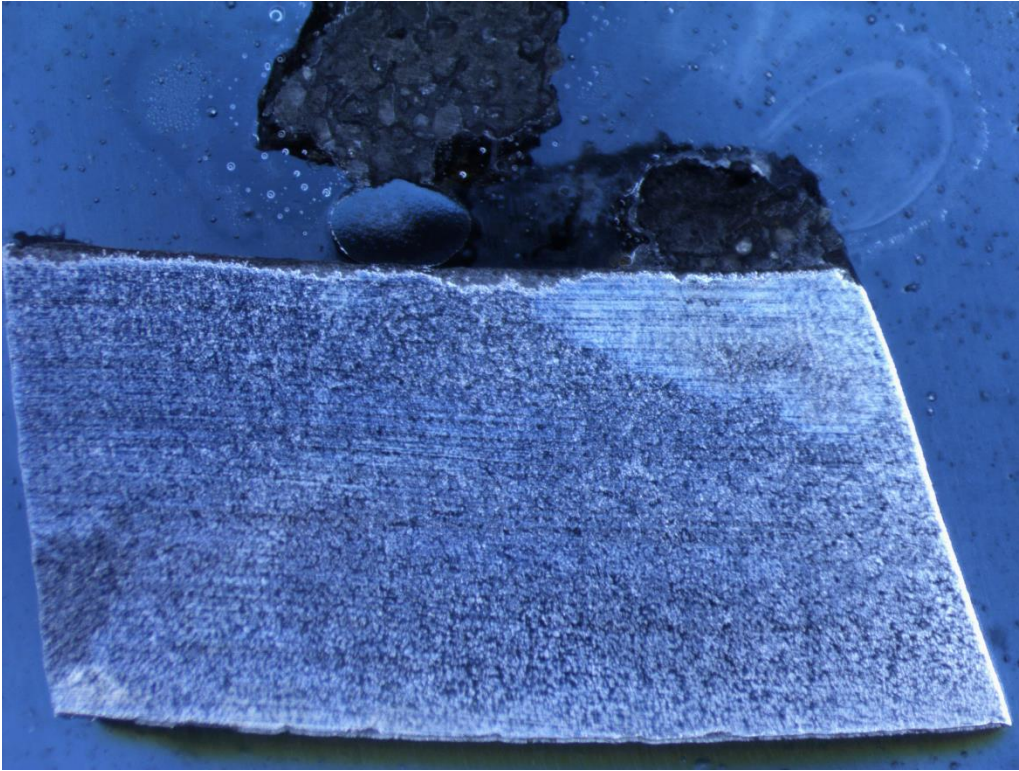
7x view of the cross section from sample N-10. Note there is a small amount of corrosion attack on the inside surface indicating the cement layer is no longer providing protection.
