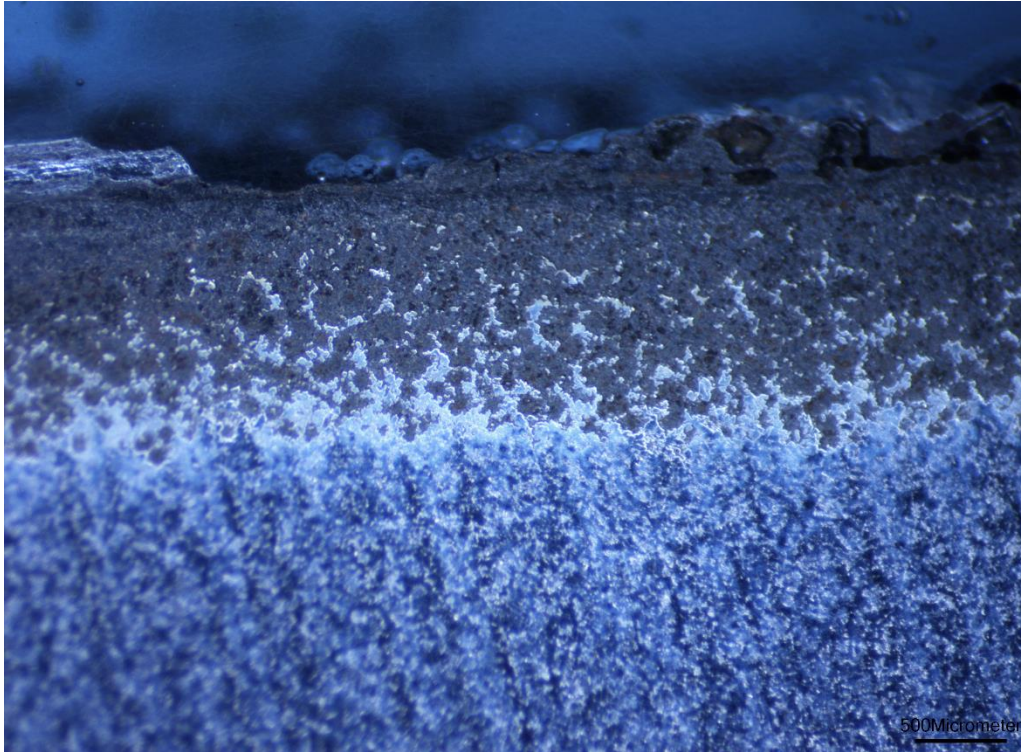
20x view of the corrosion on sample N-16.
