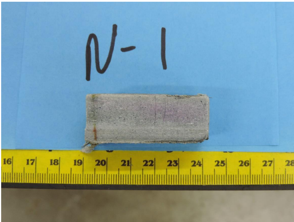
Close up of the cross section of N-1 after phenolphthalein, hardness and pH testing. This indicates that the inner layer (bottom) has a reduced pH as well as the top layer.
