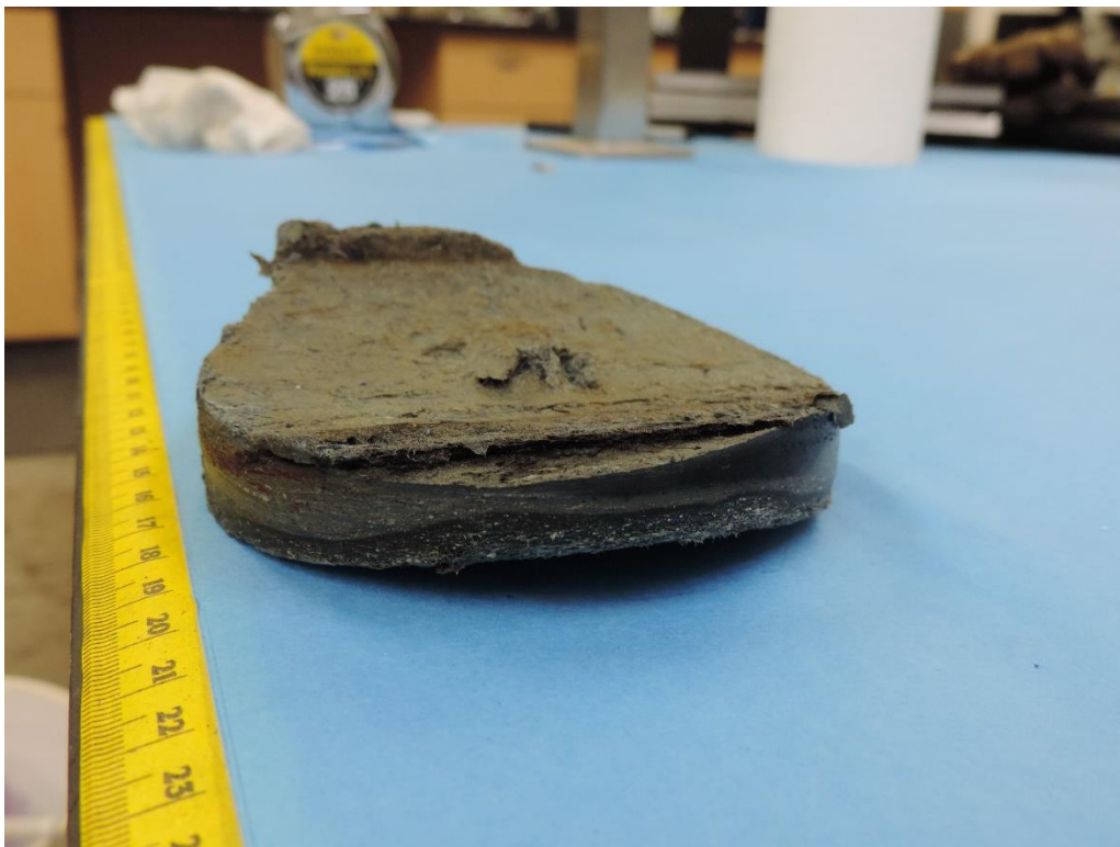
Close up of an area of delamination and thinned wall thickness on sample N-6.
