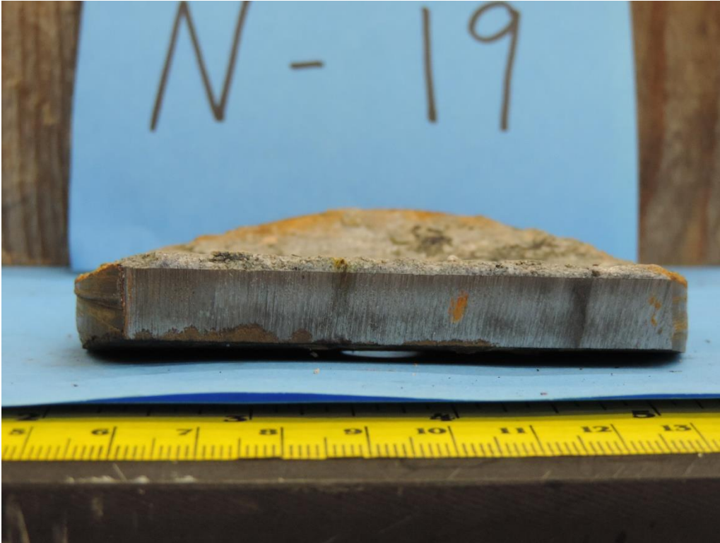
Cross section of sample N-19 after pH and phenolphthalein testing. This indicates that the upper layer of cement is slightly acidic trending toward neutral close to the cast iron.
