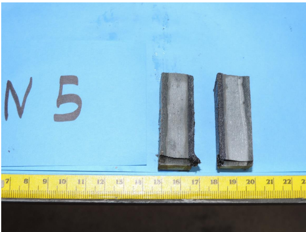
Close up view of the cross sections of sample N-5. Note the layers of attack are clearly visible at the inside and outside of the sample.
