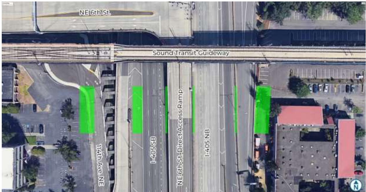
Figure 62: Permitted area (highlighted in green) of falsework and temporary support structures (photo credit to Google Earth).
