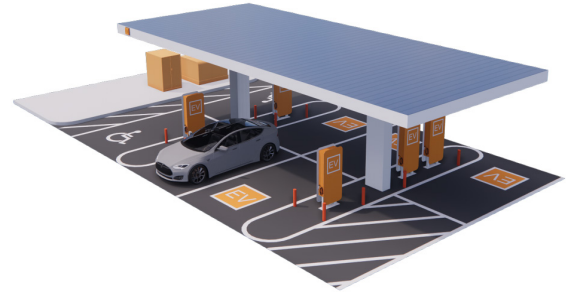
Figure 11. Example of DC Fast Destination Charging
