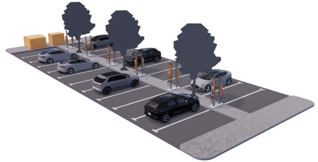
Figure 10. Example of Level 2 Destination Charging
