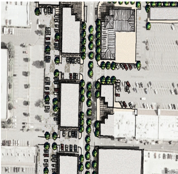
This illustration of a future, “walkable” Factoria illustrates the use of parking access streets between buildings that are located along Factoria Boulevard. These streets provide drivers with an indication that parking is available in front of stores, and provides a route to the parking behind buildings. With a double loaded parking configuration, these buildings should be 75-80 feet apart.
