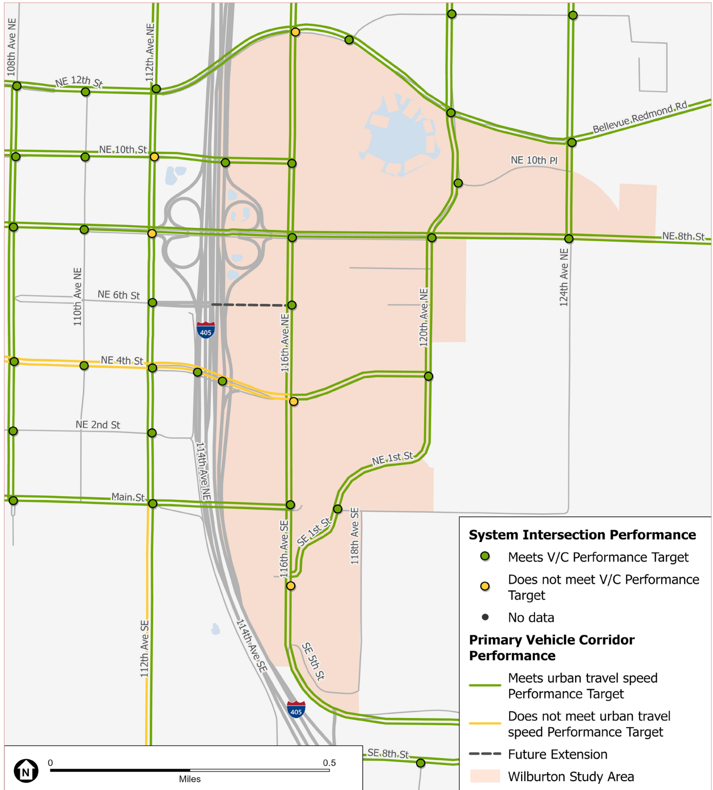
FIGURE 4 Primary Vehicle Corridor System Intersection and Speed Performance - 2044 Growth Alternative in the Wilburton Study Area Vicinity
