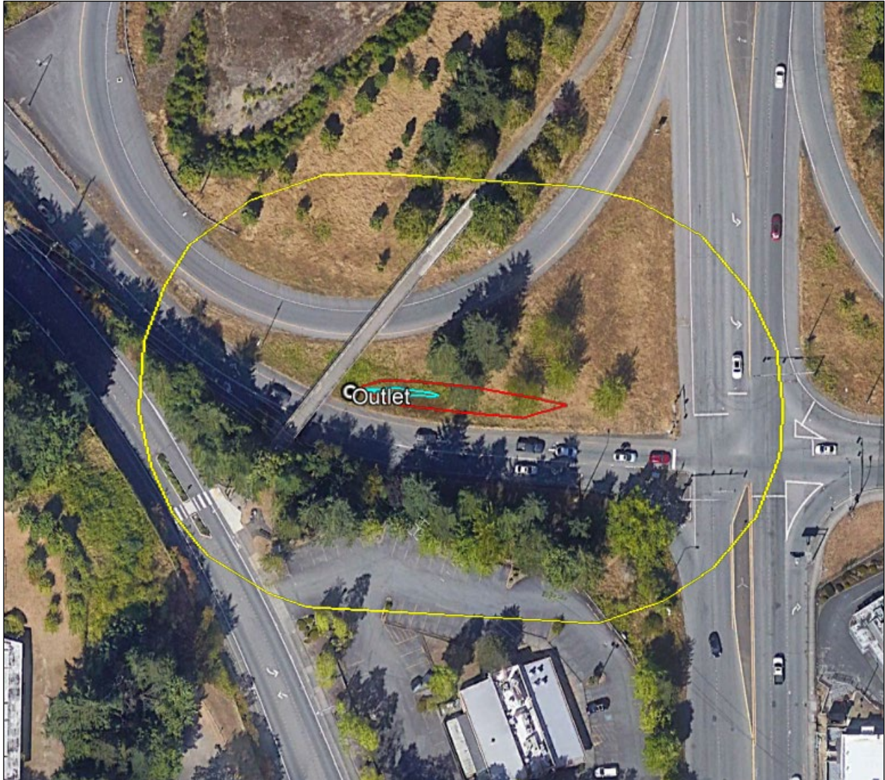
Figure 1. Detail of Cowardin Classes for Wetland W1 (red outline is the wetland and yellow is 150-foot boundary). Hydroperiods are seasonal ponding near the outlet in blue, while the remaining wetland is saturated.
