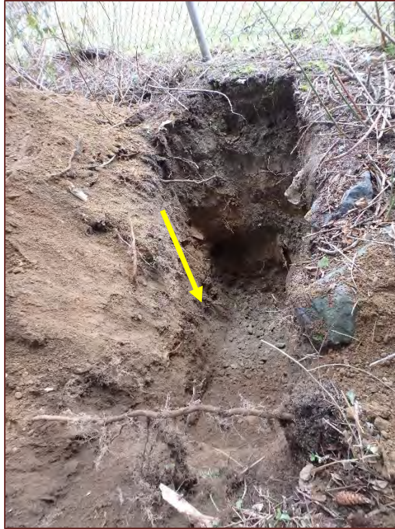
Contact of Cover Soil and Native Glacial Till Soils
