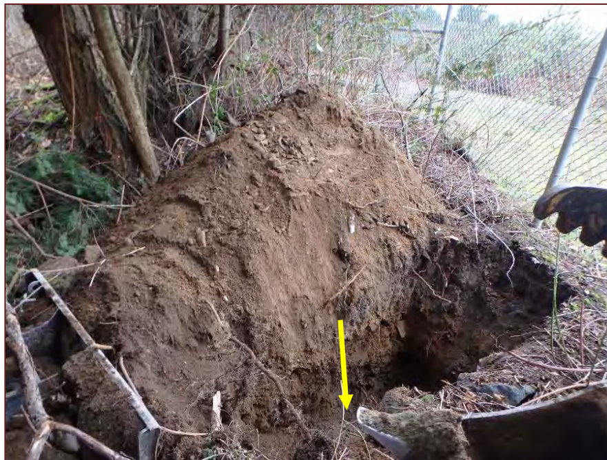
Contact of Cover Soil and Native Glacial Till Soils
