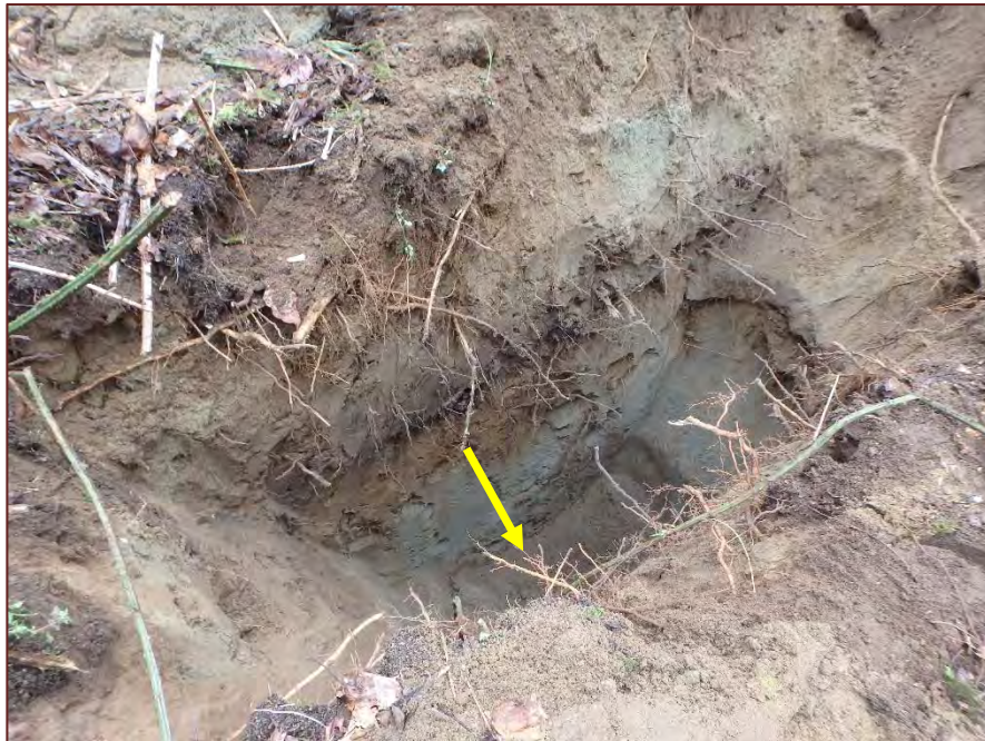
No Waste – Contact of Fill/Outwash and Native Glacial Till Soils
