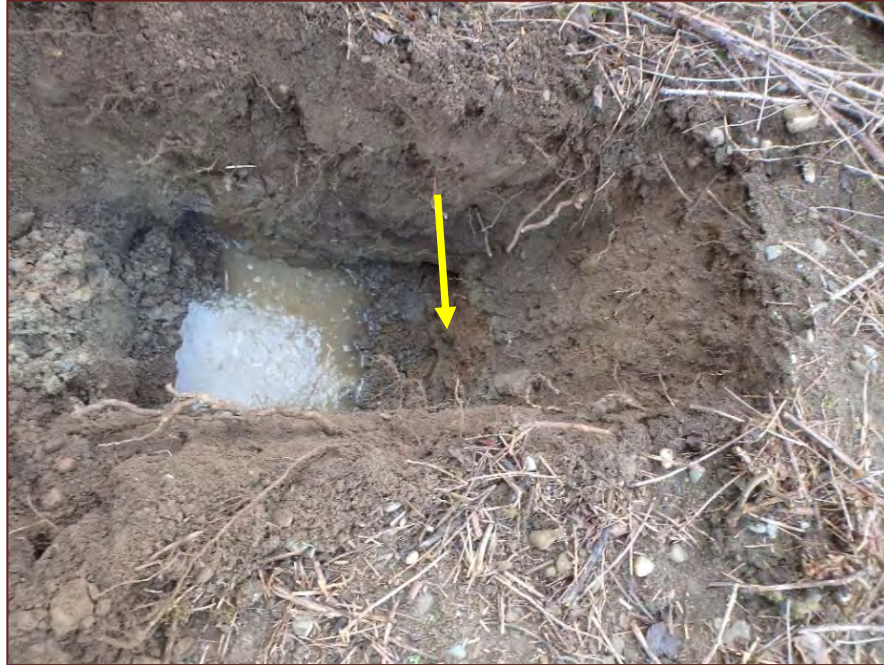
Seepage at Contact with Landfill Debris and Native Glacial Till Soils
