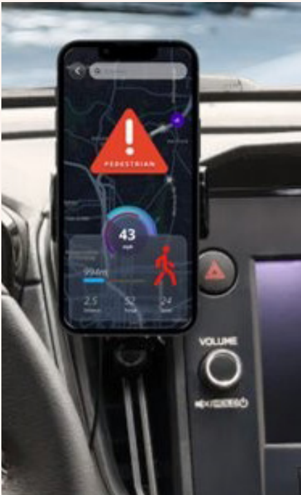
Figure 8: An example safety notification from the C-V2X pilot.
