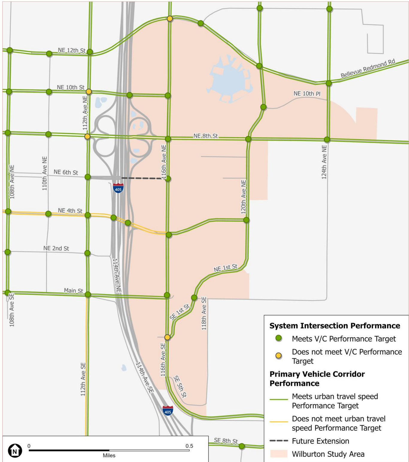
FIGURE 11-34 Primary Vehicle Corridor System Intersection and Speed Performance - No Action Alternative in the Wilburton Study Area Vicinity
