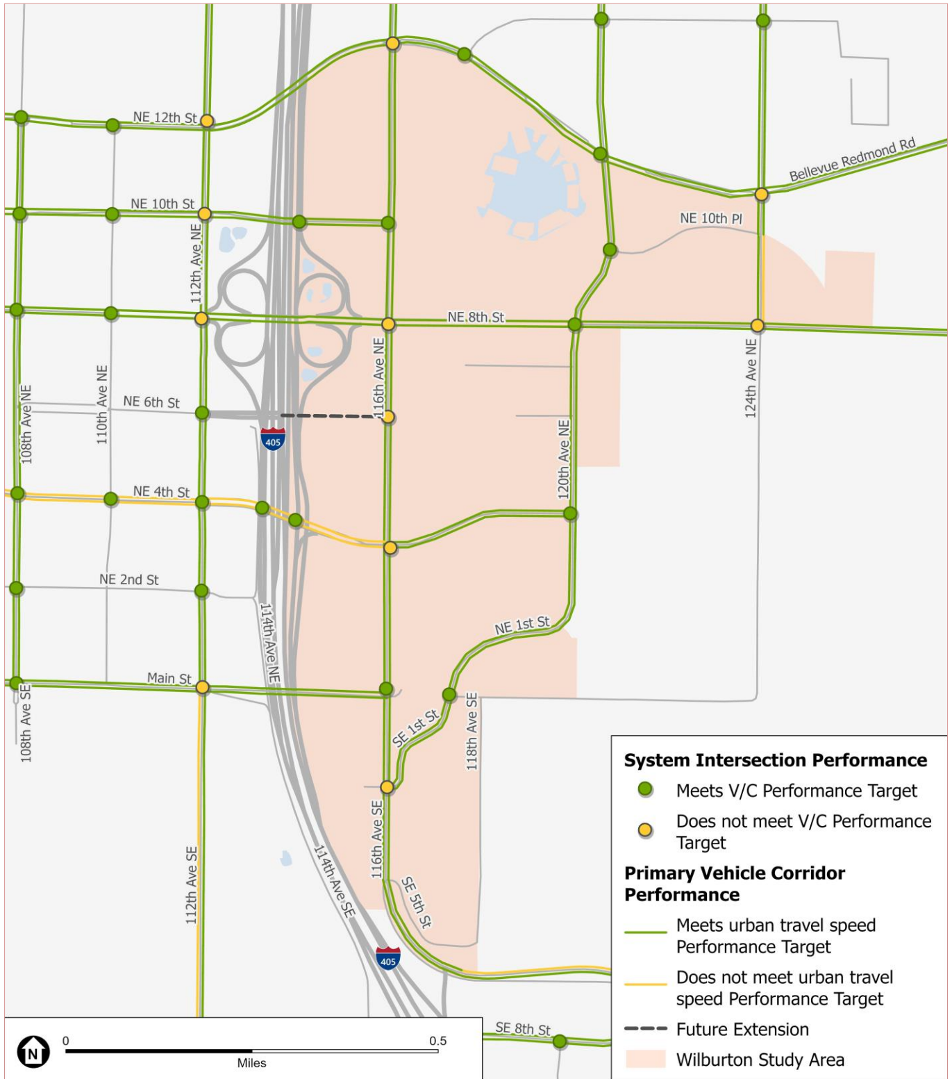
FIGURE 11-46 Primary Vehicle Corridor System Intersection and Speed Performance - Alternative 3 in the Wilburton Study Area Vicinity
