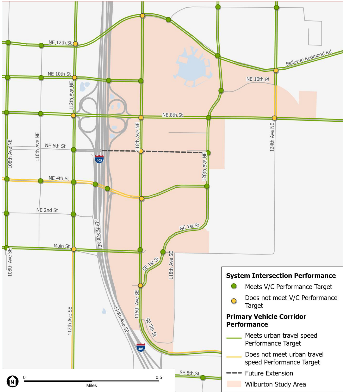
FIGURE 11-47 Primary Vehicle Corridor System Intersection and Speed Performance - Alternative 3A in the Wilburton Study Area Vicinity
