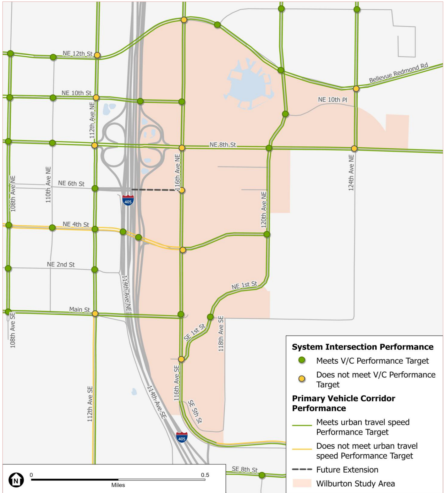
FIGURE 11-42 Primary Vehicle Corridor System Intersection and Speed Performance - Alternative 2 in the Wilburton Study Area Vicinity
