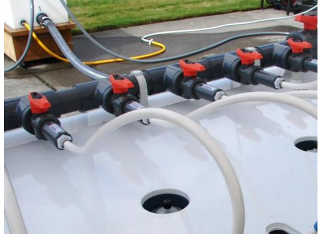
Piped Manifold Connected to Portable Blivet
