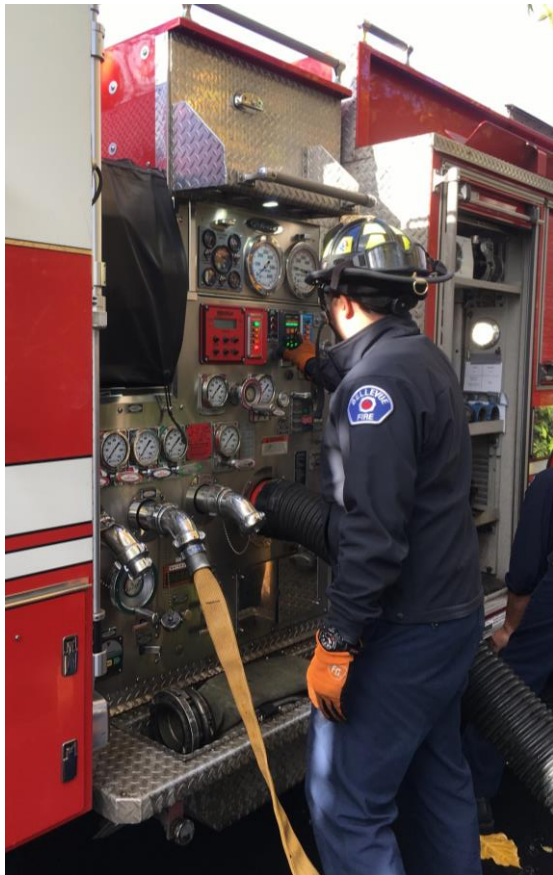
Fire Truck Drafting Operation with Suction (Black) and Discharge (Brown) Hoses
