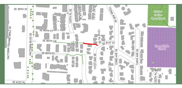
Description: This project would install approximately 130 feet of timber staircase along the paved trail between 131st Ave SE and 131st PI SE west to 129th PI SE, approximately 420 feet (210 feet per side) of pedestrian railing on both sides of the trail, and directional bollards at both entrances of the trail within the street limits included in this description. Proposed locations are estimated locations and are subject to design engineering guidelines.
