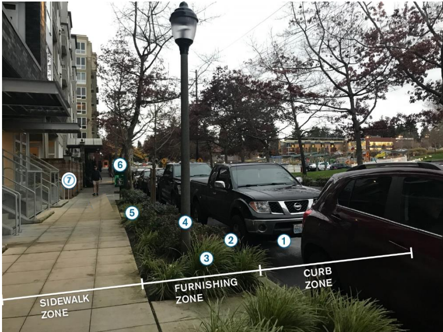
Figure 11 Residential Mixed Use: NE 1 st Street
