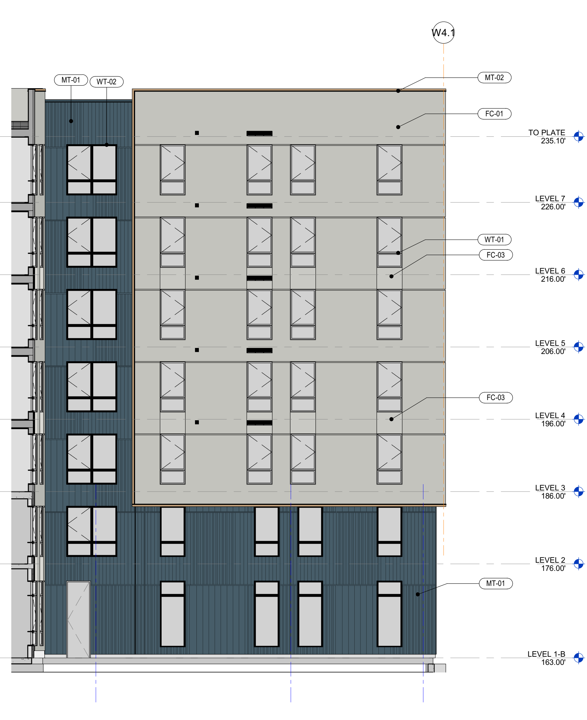
A3 COURTYARD WEST ELEVATION - COLOR 1/8" = 1'-0"
