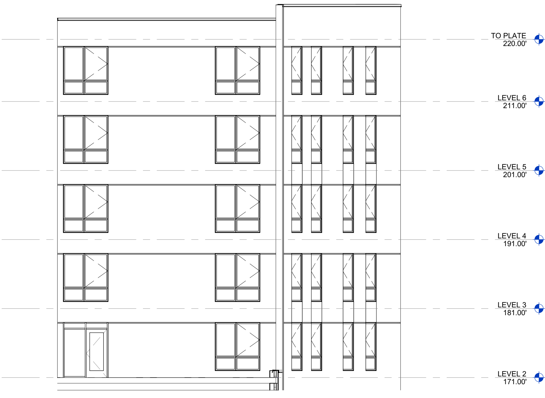
D1 TERRACE NORTH ELEVATION 1/8" = 1'-0"
