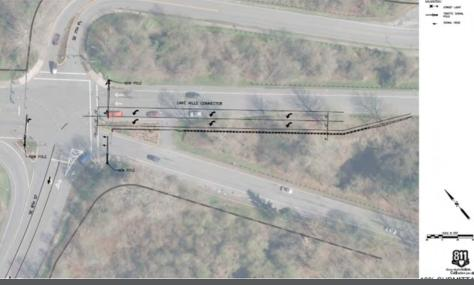
Figure 44: City of Bellevue planned Improvements Lake Hills Connector at Southeast Eighth Street Signal Upgrade.
